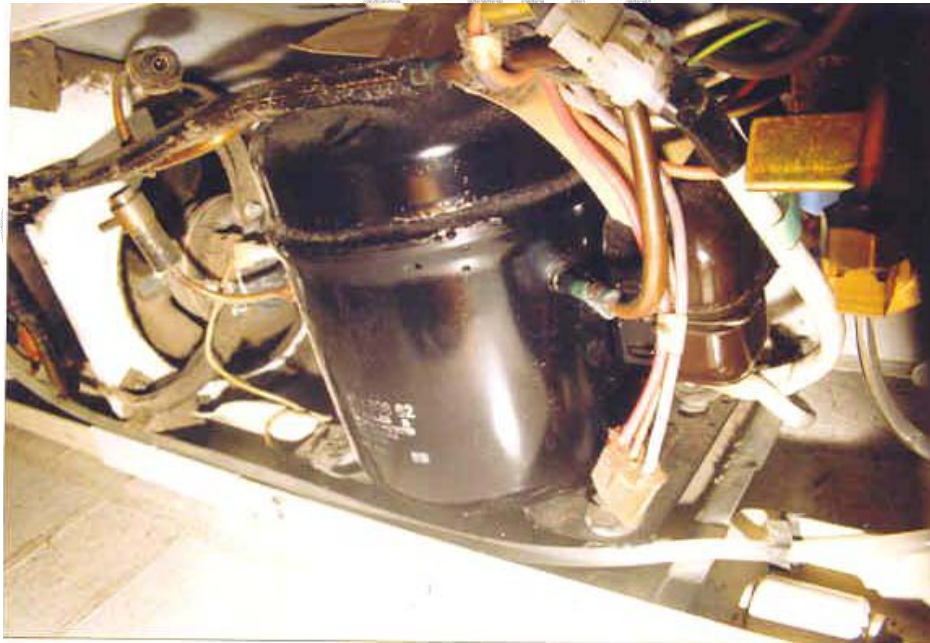
Fig071_06 Typical Compressor Jammed Under A Refrigerator
