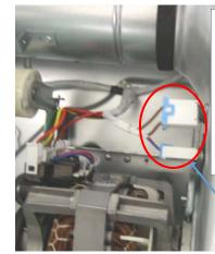
**New Version of** Blower Housing, it may be necessary to separate the harness wrap on replacement housing. Please maintain shielding on the low voltage wires.
