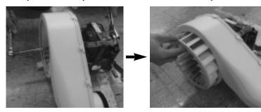
4. Dismantling of case fan: Remove 3 screws.
