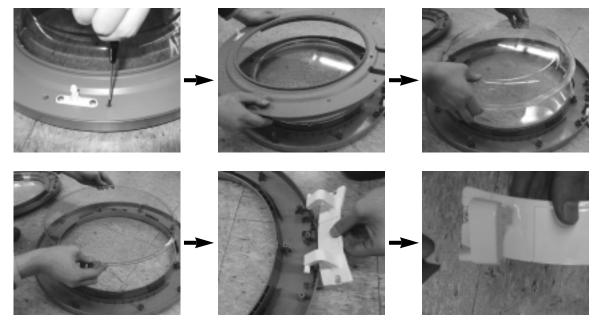
3. Door lock ass'y: Separate door lock ass'y after removing 2 screws.
