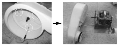
5. Dismantling of bracket motor: Remove 2 clamp motors each.
