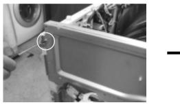
2. Remove 2 screws from left and right at the top.
