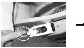
3. Separate humidity sensor connector.
