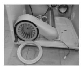
(7) Remove the cover fan and 3 screws.
