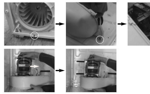
2. Separation of cover fan: Remove 2 screws.
