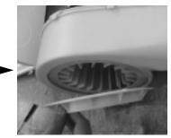
3. Separation of impeller fan: Fix motor axis and separate fan.
