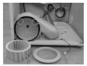
$(\underline{8})$  Remove the 4 screws and the motor ass'y.
