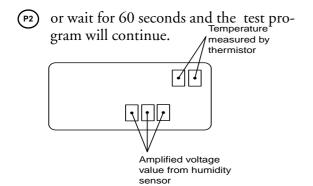
The program heats, increasing the temperature by 14° in max. 10 minutes, then allows it to cool for 5 minutes (testing that the heating element is working).
