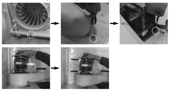
2. Separation of cover fan: Remove 2 screws.
