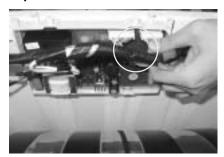
3. Separate humidity sensor connector.
