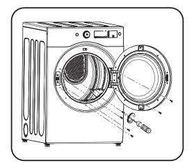
2. Then remove the door out of the front cabinet as indicated by the arrows.
