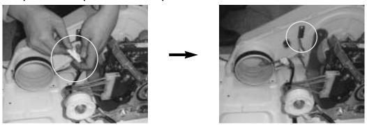
2. Separation of thermostat fan: Separate connector. → Remove 2 screws.
