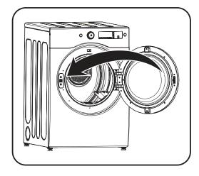
6. Secure the hinge using the bolts you removed in step 1.
