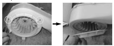
3. Separation of impeller fan: Fix motor axis and separate fan.
