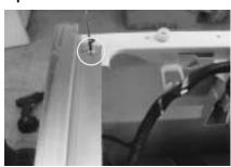
3. Separate frame upper after removing harness at the back.
