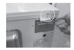
3. Separate plate top by pushing it at the front part in the direction of arrow.
