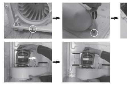
2. Separation of cover fan: Remove 2 screws.
