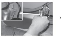
3. Remove duct outlet F in the direction of  $\rightarrow$
