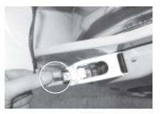
3. Separate humidity sensor connector.
