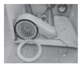
8 Remove the 4 screws and the motor ass'y.
