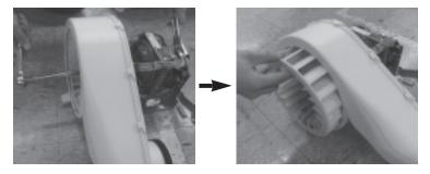
4. Dismantling of case fan: Remove 3 screws.
