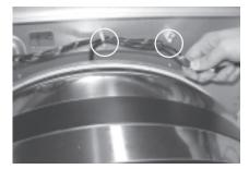
2. Remove 2 screws from left and right at the top.
