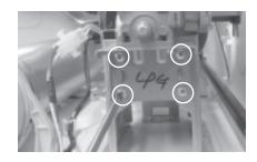
3. Remove 2 screws and separate igniter connecter.
