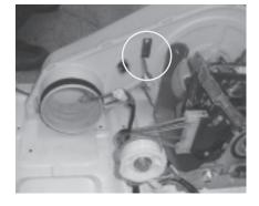
2. Separation of thermostat fan: Separate connector.  $\rightarrow$  Remove 2 screws.
