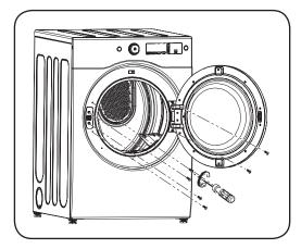
2. Then remove the door out of the front cabinet as indicated by the arrows.
