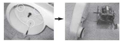
5. Dismantling of bracket motor: Remove 2 clamp motors each.
