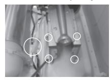
3. Remove 2 screws after removing harness at thermostat Cut-Out, Hi-Limit.
