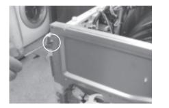
3. Separate frame upper after removing harness at the back.
