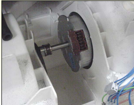
Exposed drum drive motor
