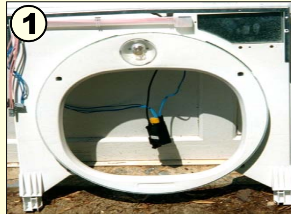
Frame with fascia, front & side panels removed.
