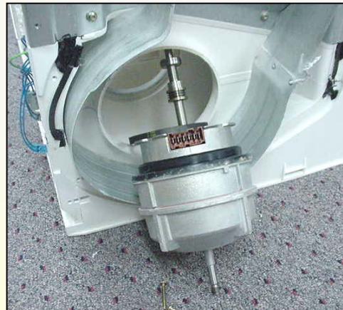
Disassembled drum drive motor
