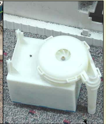
Remove drain pump
