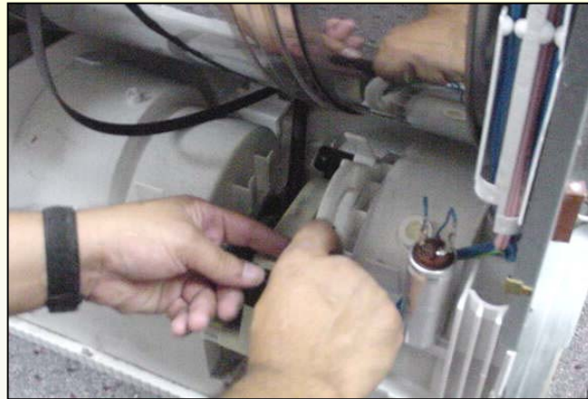
Slide drive belt off pulley
