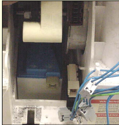
Disconnect motor wires
