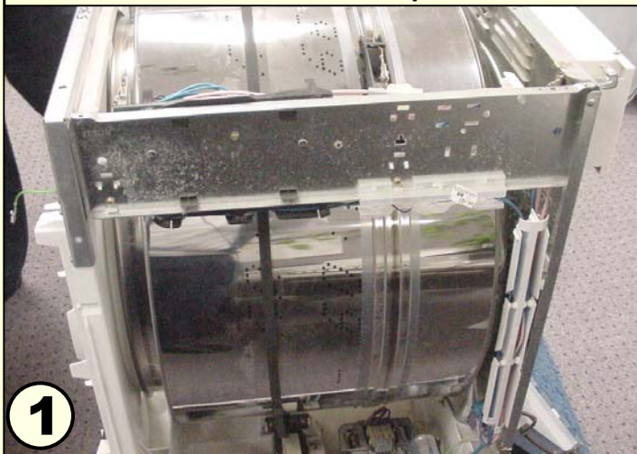
Frame with fascia, front & side panels removed.
