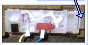
**NOTE:** The white plastic linkage 1st opens the detergent dispenser door, then cocks in place to dispense rinse-aid when the wax motor operates the 2nd time. After the 2nd operation, the linkage resets for the next wash program.
