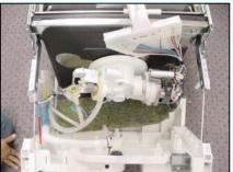
Pull wires from J-box Pull out sump hose
