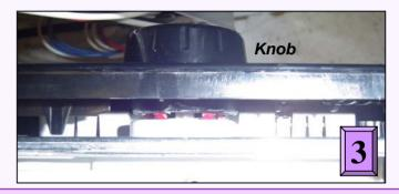
Inserting knob shaft into module
