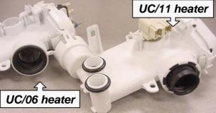
HINT: Don't use softer bearing heater assemblies (UC/11 & later) on older UC/06 models since sump, circulation pump, base and heater clamps/gaskets have to be replaced as well for heaters to fit.
