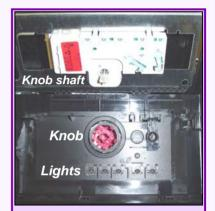
Inside of fascia panel and front of control module showing knob shaft & rear of knob
