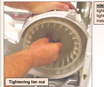
HINT: Make sure fan is tight. If fan nut won't tighten down adequately, install a lockwasher.
