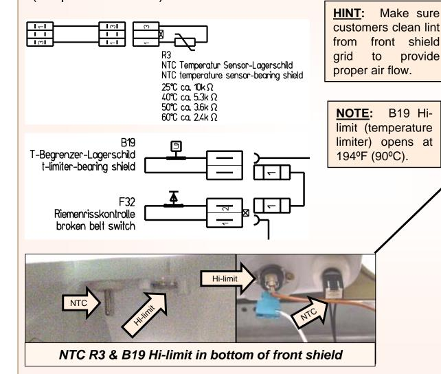
**NOTE:** Fault codes E:01, E:11 & E:12 occur when lint screens are clogged. Control module reads NTC and approximates air flow – when air flow is too low, fault codes are generated. B19 Hi-limits do not generate fault codes.
