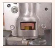
For best results, fan must be running and burner air holes must be clear.
