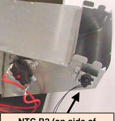
NTC R2 (on side of electric heater housing)
