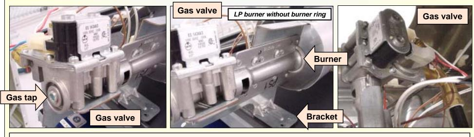
Gas valves (3 screws) and burners (2 screws) are attached to the same gas valve/burner mounting bracket. Brackets are held to dryer bases by 2 screws (@ front of gas valves & rear of burners) & to burner chambers by one screw.
