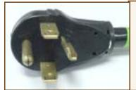
HINT: Canadian dryers use a NEMA 10-30P 240V, 30A, 4-wire plug, which mates to a NEMA 10-30R outlet (receptacle).
