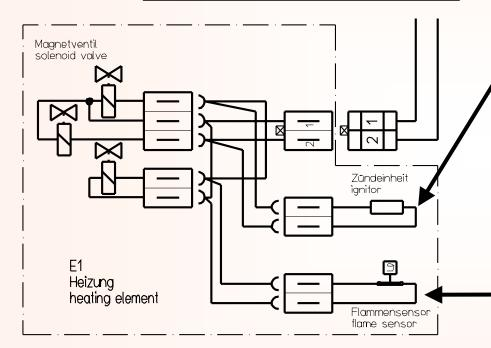
**NOTE:** Sensors react to flame out in less than 45 seconds. The flame sensor, located in the front of the burner assembly (near the burner & igniter), reliably reignites natural gas & LP flames should they ever go out.
