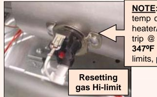
**NOTE:** Hi-limits (high temp cutouts), located on heater/burner housings, trip @ **347°F (electric)** or **347°F (gas)**. To reset Hi-limits, press **red** button.
