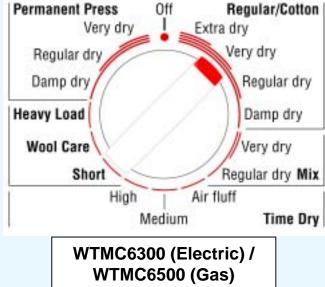
**HINT:** Electric dryers can be run on 240V **or** 208V. To change voltage from 240V to 208V, use voltage changeover test (8<sup>th</sup> position from right).
