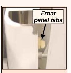
**HINT:** Front panel hangs to frame by six tabs, three per side. <u>Panels can be tricky to</u> <u>reinstall</u>, especially getting all six tabs to engage frame.
