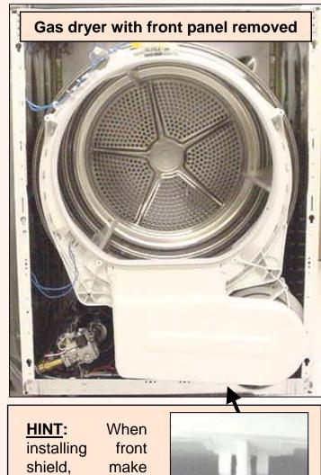
**HINT:** When installing front shield, make sure notch on bottom is seated on frame.
