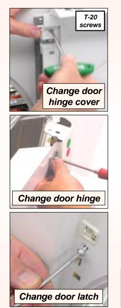
**NOTE:** Occasionally door hinge white plastic bushings can fall off. Make sure all four are collected when removing hinges.
