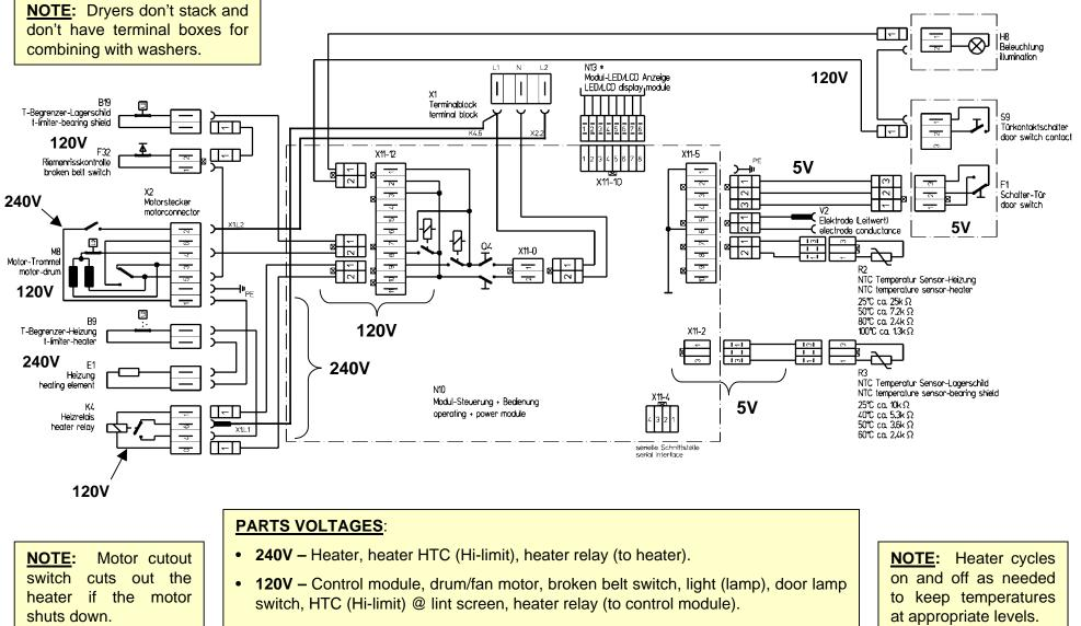
5V or less – Door switch (to control module), NTC (heater), NTC (lint screen), moisture sensor.
