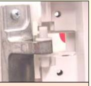
**NOTE:** Occasionally door hinge white plastic bushings can fall off. Make sure all four are collected when removing hinges.
