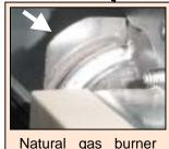
Natural gas burner ring (not used for LP)
