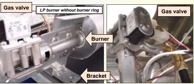
Gas valves (3 screws) and burners (2 screws) are attached to the same gas valve/burner mounting bracket. Brackets are held to dryer bases by 2 screws (@ front of gas valves & rear of burners) & to burner chambers by one screw.
