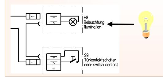
**HINT**: To access bulb, unscrew one screw in cover and pull hinged cover downward.
