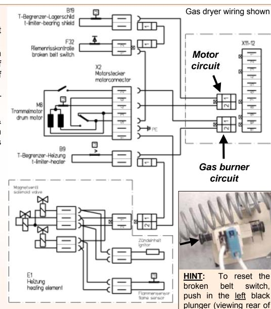
HINT: Remove rear panel to access drum drive motor, belt/pulley & electric heater/gas burner.
