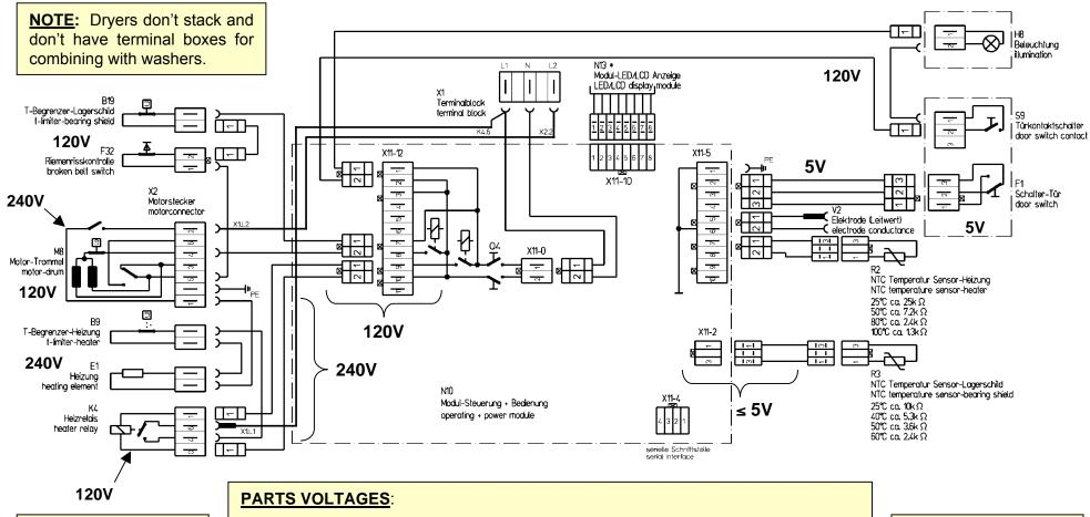
**NOTE:** Motor cutout switch cuts out the heater if the motor shuts down.
