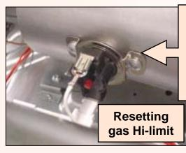
NOTE: Hi-limits (high temp cutouts), located on heater/burner housings, trip @ 347°F (electric) or 347°F (gas). To reset Hilimits, press red button.
