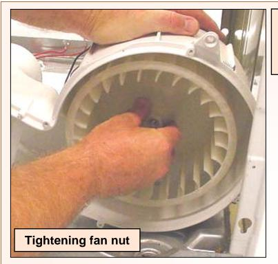
**HINT:** Make sure fan is tight. If fan nut won't tighten down adequately, install a lockwasher.
