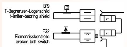
NOTE: Fault codes E:01, E:11 & E:12 occur when lint screens are clogged. Control module reads NTC and approximates air flow – when air flow is too low, fault codes are generated. B19 Hi-limits do not generate fault codes.
