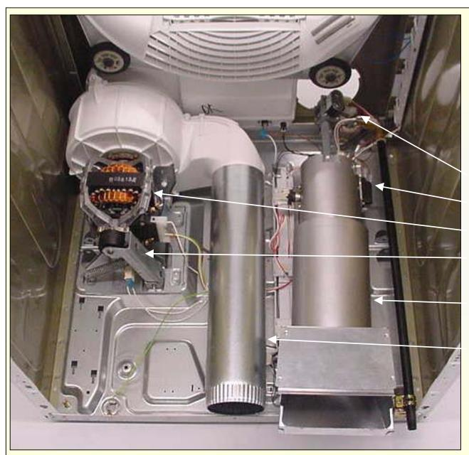
Gas dryer after drum has been removed.
