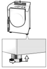
The dryer should be level with all four feet firmly on the ground. The dryer must not wolbble. If the dryer is not level or if it does wolbble, the feet must be adjusted. Adjust the height-adjustable feet until the dryer does not rock and is level, both front-to-back and side-to-side.
