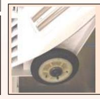
HINT: Reconnect drum belt <u>after</u> front panel installation so drum (& support wheels) won't be in tension. After belt installation, reset broken belt switch.
