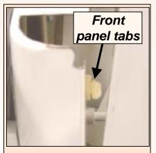
HINT: Front panel hangs to frame by six tabs, three per side. Panels can be tricky to reinstall, especially getting all six tabs to engage frame.
