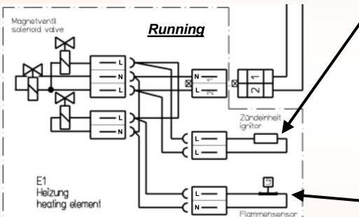
NOTE: Sensors react to flame out in 30 - 60 seconds.
