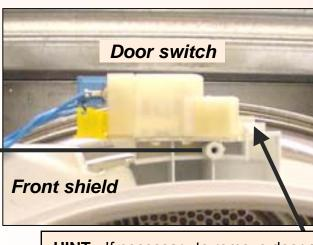
**HINT:** If necessary to remove door switch, push onto latches (at both ends) and slide switch toward rear of front shield.
