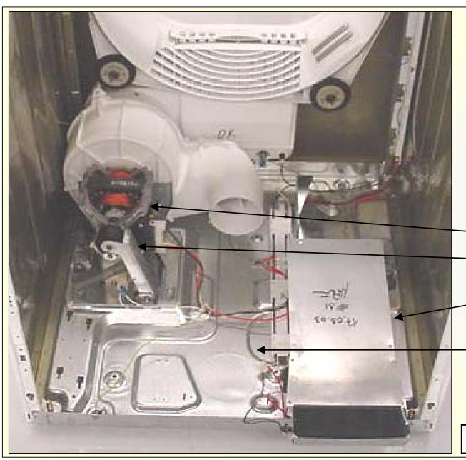
Electric dryer after drum has been removed.
