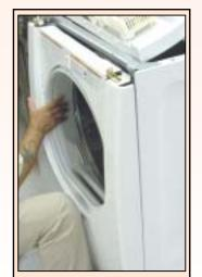
HINT: When aligning front panel tabs on frame, make sure door seal is seated properly.
