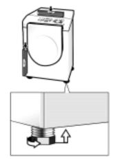
The dryer should be level with all four foat firmly on the ground. The dryer must not wobble. If the dryer is not level or if it does wobble, the feet must be adjusted. Adjust the height-adjustable feet until the dryer does not rock and is level, both front-to-back and side-to-side.
