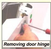
HINT: To remove door, open it 180° (so it doesn't fall off), remove hinge cover and lift door off hinge.
