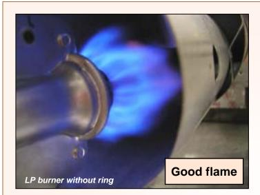
Good flame – fan pulls air through burner cavity and air flows freely through burner air holes. Flames are blue, compacted and uniformly distributed – flames have "roaring" sound.
