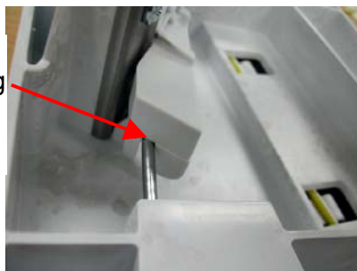
No gap between linkage and moulding at this point
