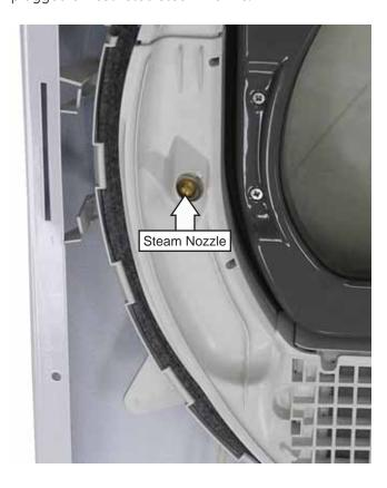
The steam nozzle can be replaced without disassembly of the dryer. Replacement can be performed by opening the dryer door to access the steam nozzle. A 7/16" or 11-mm nut driver can be used to unscrew the nozzle from the air duct assembly.
