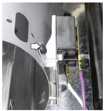
5. Remove the flame detector from the tab at the bottom.
