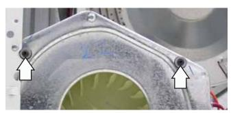
10. Remove the Phillips-head screw, then disengage the motor moisture shield from the motor bracket.
