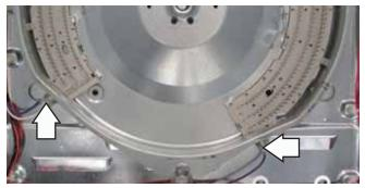
3. Bend back the single metal tab on the housing holding the heater in place.
