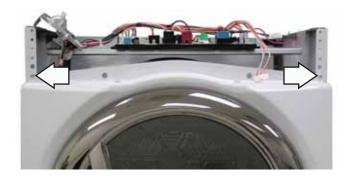
8. Tilt the top edge of the front panel out and press on the John Guest connector collar to release the water line.
