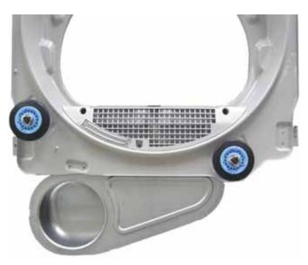
Each roller is part of an assembly that consists of a roller, roller shaft, 2 plastic triangular clips, 2 washers, and a 17-mm hex nut.
