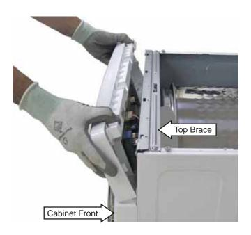
4. Disconnect the control panel wires and harnesses.
