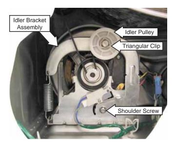
When removing the idler bracket, it is first necessary to release the belt from the idler pulley (See *Drive Belt.*), and disconnect the spring from the idler bracket.
