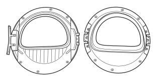
6. Lift and rotate the window assembly 180° and replace. Also rotate the inner face 180° and replace.
