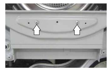
7. Lift the filter guide and inlet from the drum support.
