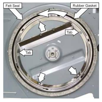
4. At each tab location, pull the rubber gasket away from the circular bracket.
