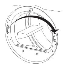
10. Move the mounting screw to the upper screw hole position on the hinge so that the door can be set on the cabinet during final installation.
