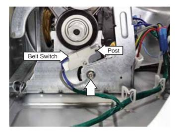
4. Disconnect the wire harness from the belt switch.
