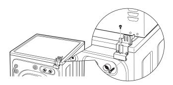
8. Lift the dryer on top of the washer. Protect the washer control panel with cardboard or other protection. Be sure to lift the dryer high enough to clear the washer control panel.
