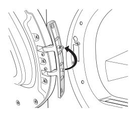
11. Fasten the hinge back on at the top and bottom with the hinge mounting screws.
