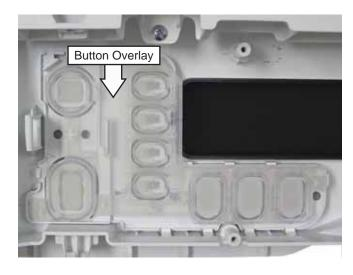
7. Carefully peel back the button overlay and remove it from the control panel.
