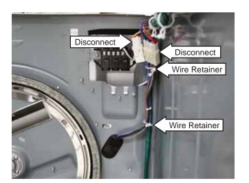
5. From the rear of the cabinet, peel back the wiring grommet from the wiring entry opening.
