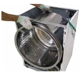
The drum shaft is permanently attached to the back of the drum. A plastic washer is installed on the drum shaft.
