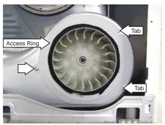
**Note**: In the following step, to prevent the blower wheel from turning while removing the center nut, apply a 7/8-in. wrench to the nut on the end of the drive motor shaft as shown below.
