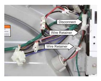
3. From inside the dryer, starting at the pointed location, carefully peel up the flexible housing and pull the assembly thru the opening in the drum support.
