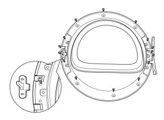
9. Remove the female end of the latch from the front panel of the dryer, rotate 180°, and replace on the opposite side.
