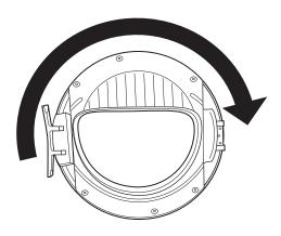
7. Replace a door screw in the center of the side opposite the hinge. Then put the male end of the latch into place and fasten with two door screws.
