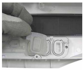
8. Release the 11 tabs that attach the button frame to the control panel, then lift the frame from the panel.
