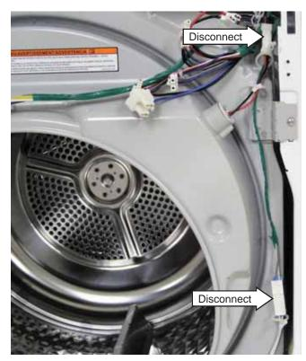
3. Remove the disconnected touch sensor wire harness from the 2 top front wire retainers.
