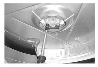
**Note:** Do not lose the grounding ball or the tinnerman mounting clip from the rear of the dryer.
