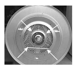
The air passes through the drum, picking up moisture and is drawn through the lint filter into the ductwork at the front of the dryer.
