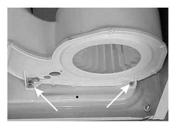
5. Remove the front motor lock by inserting a screwdriver at the rear of the housing to release the housing from the motor.
