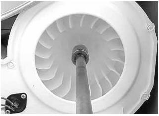
4. Remove (2) screws holding the housing to the dryer base.
