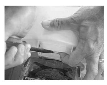
6. Raise the front of the motor and pull the housing forward.
