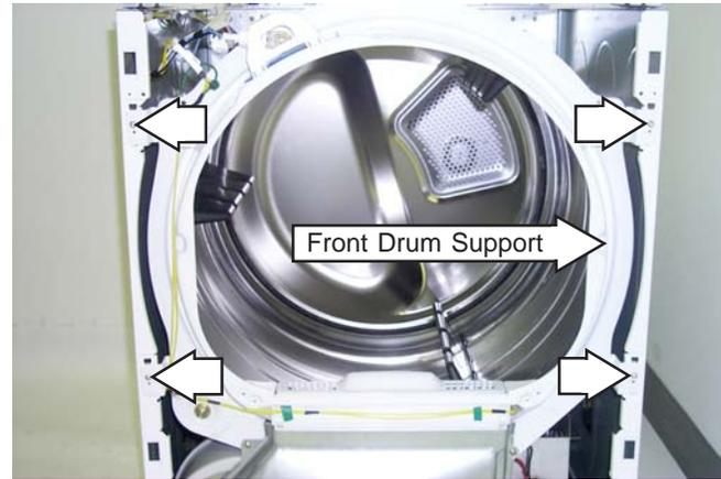
5. Grasp the top outside edges of the front drum support and unsnap the 4 corners from the sides of the dryer. Remove the front drum support.
