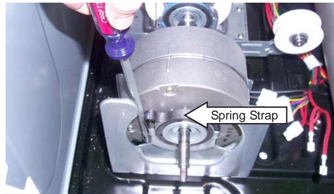
11. Remove the spring straps. Remove the drive motor from the motor bracket.
