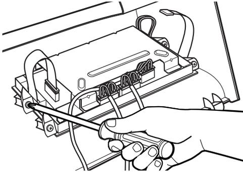
21. Place the gray wire from the serial port under the strain relief of the new backsplash.
