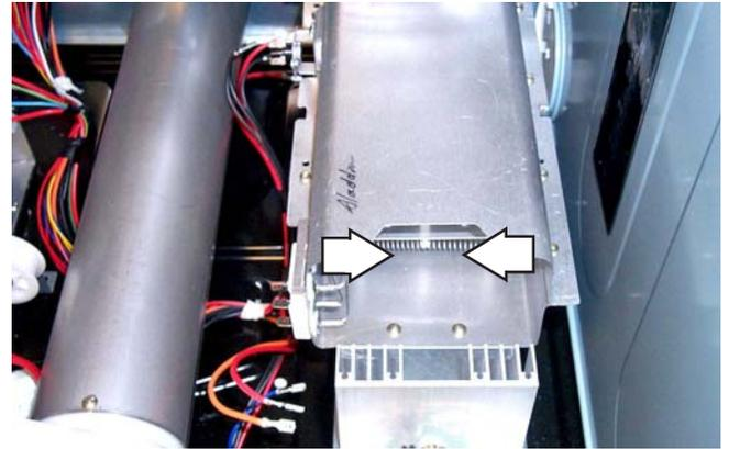
4. Remove the heater assembly.
