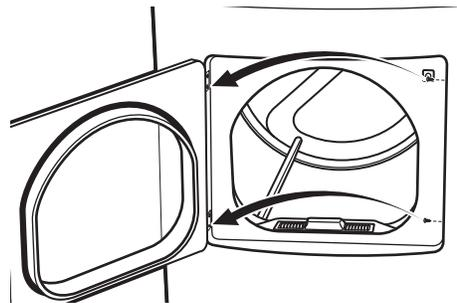
13. Tighten the two top screws of each hinge. Reinsert the plastic plugs on the side from which the door was removed.
