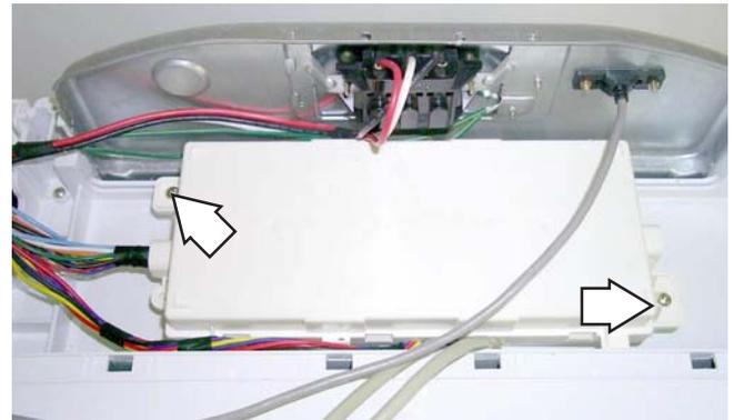
3. Slide the inverter box toward the rear of the dryer and lift out.
