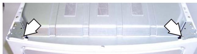
4. Lift and tilt the front panel forward slightly to disconnect wiring to the door switch.
