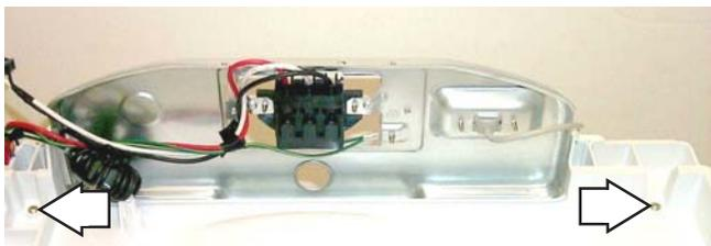
6. Lift the top cover and slide it forward to clear the front tabs.
