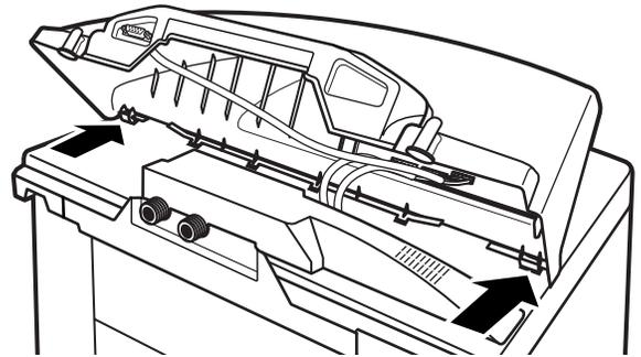
23. Secure the new backsplash to the washer using the 2 screws removed earlier.
