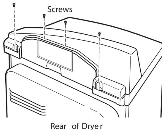
18. Attach the washer control board to the new backsplash by replacing the four screws removed from the washer control board earlier.
