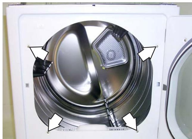
3. Remove the 2 Phillips screws that hold the front panel to the inner top cover.
