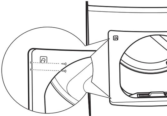
3. With the door completely open, remove the bottom screw from each hinge on the dryer face.
