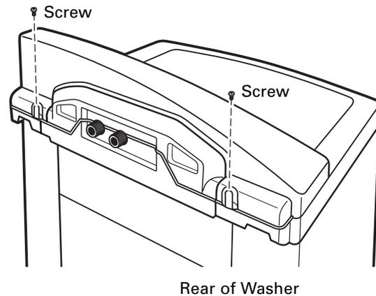
4. Remove the 2 screws holding the backslash to the rear cover. Remove the backslash from the rear cover.
