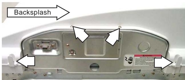
2. Place a towel over the lid of the dryer to prevent scratches to the surface. Gently lift each corner of the backslash; then roll it forward so it rests on top of the dryer.
