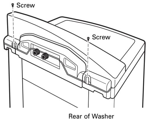
20. Secure the new washer backsplash to the rear cover using the 2 screws removed earlier.
