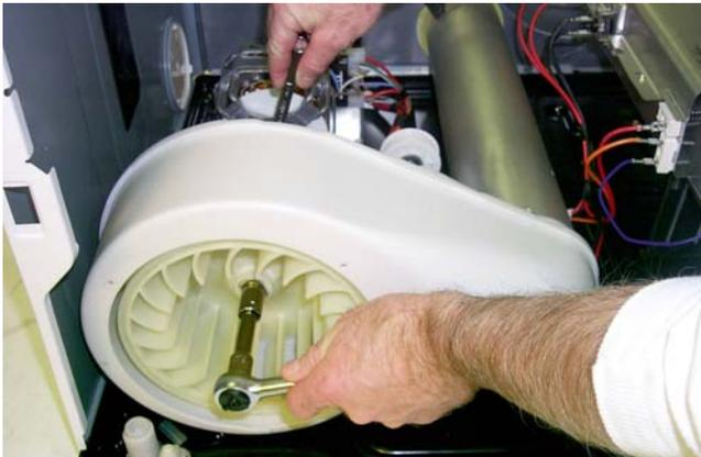
7. Remove the 3 Phillips head screws from the center of the blower housing. Remove the front screw from the dryer base.
