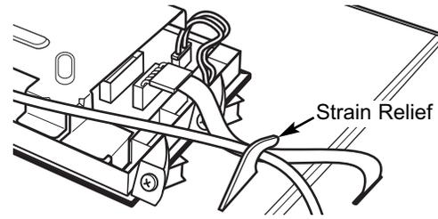
13. Attach the dryer control board to the new backsplash by replacing the four screws removed from the dryer control board earlier.
