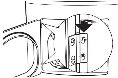
12. Remove the remaining screws from the side of the opening from which the door was removed. With these screws, secure each hinge at the bottom.
