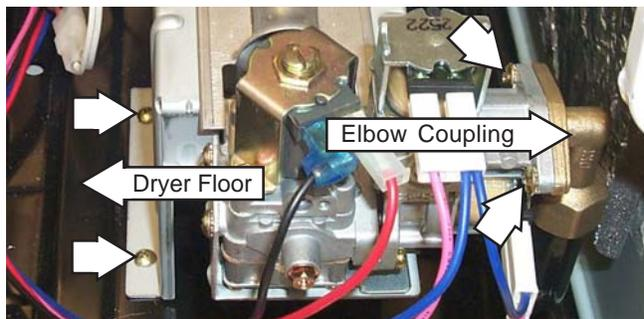
6. Slide the gas valve assembly out through the front of the dryer cavity.
