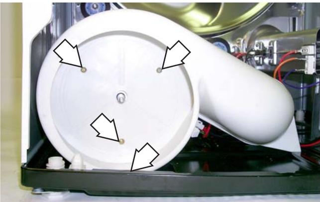
8. Remove the remaining 2 Phillips head screws from the dryer base and exhaust duct.
