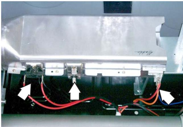
3. Remove the 2 Phillips head screws that hold the heater assembly in place.
