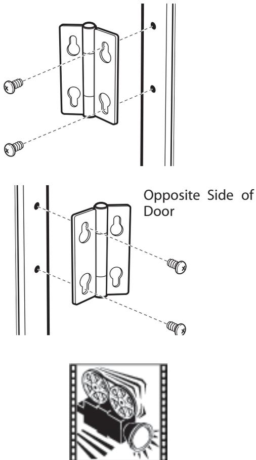
11. Insert the door on the opposite side of the opening by moving the door **IN** and **DOWN** until the top hinge and the bottom hinge are resting on the top screws.
