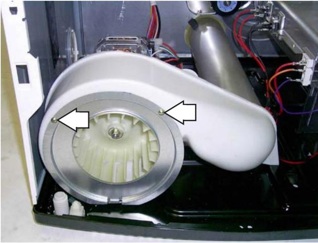
6. Remove the 13 mm center nut. (Turn clockwise to remove.) Remove the blower wheel.
