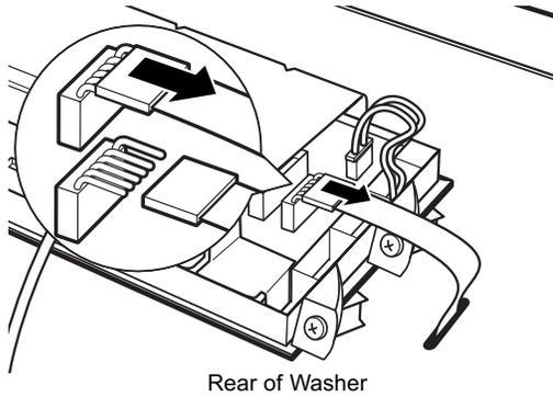
6. Remove the four screws holding the washer control board to the backslash; then remove the control board and set it aside.
