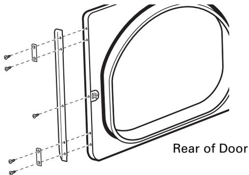
10. Remove the hinges from the door and install them on the opposite side with the hinge pin toward the outside of the door.
