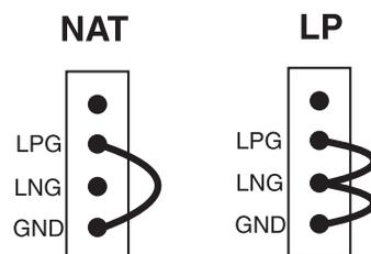
**Note:** The gas dryer main board differs from the electric dryer main board by the addition of a jumper plug on the model selector connector (the electric model has no jumper plug). Depending on how the pins have been jumped will determine what type of gas (natural or LP) the dryer is using.
