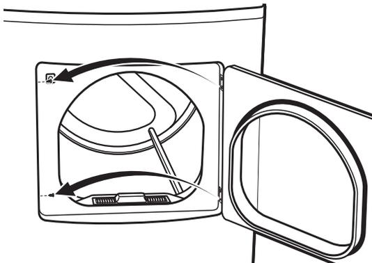
5. Loosen the top screw from each hinge on the dryer face halfway. With one hand holding the top of the door and the other hand holding the bottom, remove the door from the dryer by lifting it **UP** and **OUT**.
