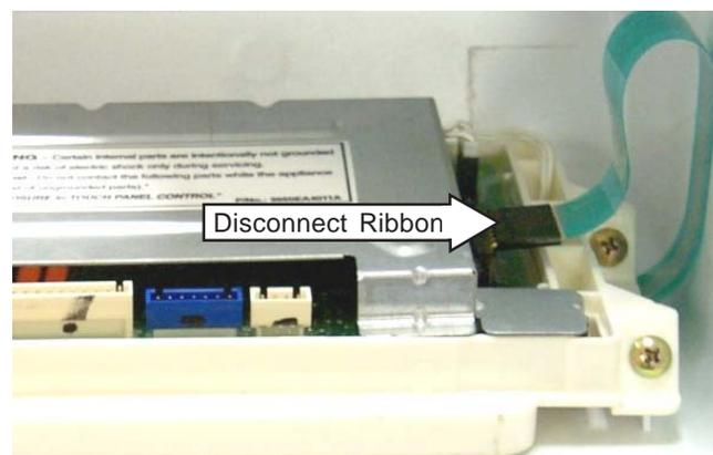
3. Remove the 4 Phillips head screws (2 on each side) that hold the main control board and LCD touch screen assembly in place. Remove the assembly.
