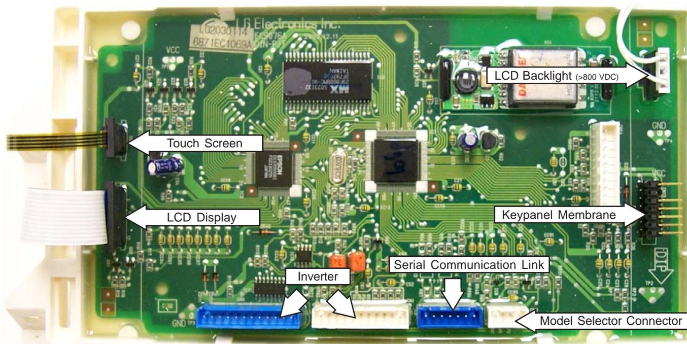
**WARNING: THE CONNECTOR AT THE LCD BACKLIGHT IS OVER 800 VDC. USE APPROPRIATE TYPE VOLTMETER OR DAMAGE COULD RESULT.**
