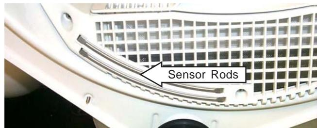
**Note:** Proper leveling of the dryer is vital for accurate sensor drying. Excessive rearward adjustment will cause clothes to tumble toward the rear of the drum, preventing contact with the sensor rods, thus producing a false dryness reading.
