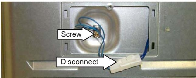
3. Remove the screw that holds the thermistor in place. Remove the thermistor.
