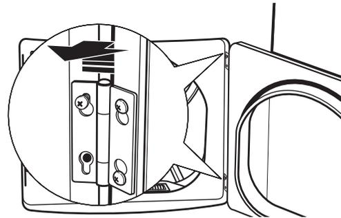
7. Remove the door catch and filler plate.
