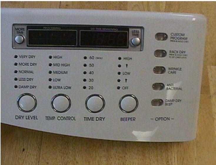
The drying cycle is shown in the left window and the time remaining is shown in the right. Feature selections like DRY LEVEL and BEEPER volume are indicated by LEDs on the panel.
