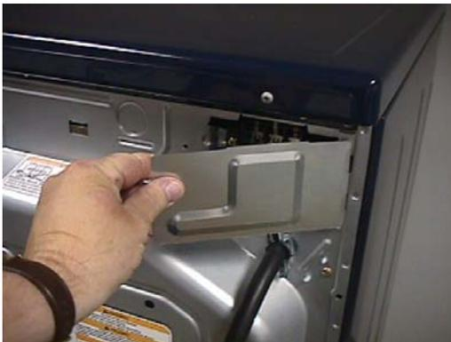
Replace the terminal block cover by inserting the tabs into the slots and letting them slide down to engage.
