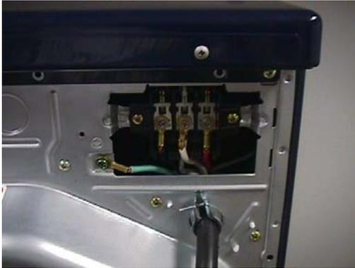
Be sure to tighten all screws firmly, but do not strip them or distort the contact area.
