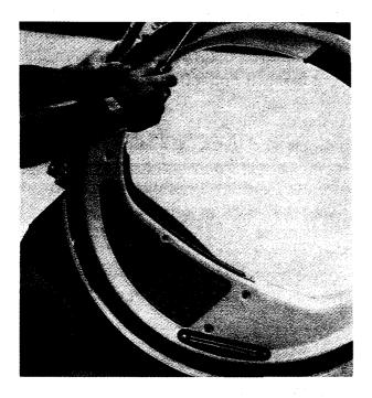
The Teflon coated side (which is the lighter of the two colors) goes against the tumbler. The seal is then looped in a "U" shape so the slot edge of the lighter colored side is to the tumbler front. Rubber adhesive is used to hold the seal overlap.
