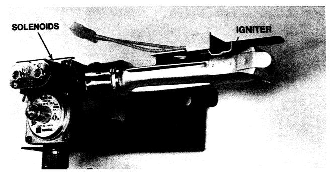
The gas controls utilize a direct ignition system (there is no pilot light). The three major components of the gas are: Igniter, Radiant Sensor and Gas Valve.
