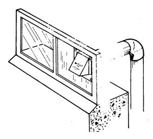
Install ductwork from the dryer to exhaust hood. All joints must be made so exhaust end of one pipe is inside the intake end of next pipe. On flexible metal ductwork, all joints should be secured with a clamp. **DO NOT** use sheet metal screws when assembling rigid ducting. These should be taped.
