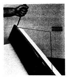
2. Tip control panel assembly forward.
