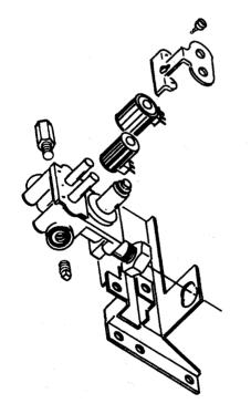
**Note:** The coil positioning tabs and matching holes in the coil holding bracket for each coil.
