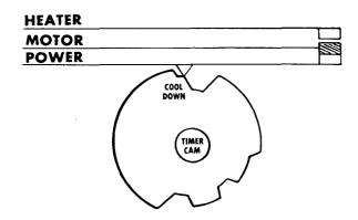
The length of the cool-down period depends upon the cycle selection. Permanent Press has an extended cooldown to lower the temperature of the garments so as to minimize wrinkling which would result from the warm garments coming to rest at the bottom of the tumbler.
