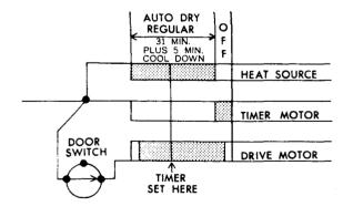
With the timer set in this position, the circuits are completed to the heat source and drive motor.
