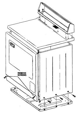
2. Lift up on front panel and swing bottom of panel away from dryer to disengage top of panel from dryer top.
