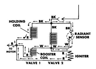
Because the secondary coil on Valve 2 is bypassed by the radiant sensor contacts, Valve 2 remains closed and prevents the release of gas.
