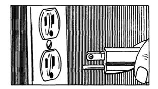
If a mating wall receptacle is not available, contact a qualified electrician to have the wall receptacle replaced. If there is any question, local building officials or electrical utility should also be consulted.
