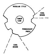
As the timer advances towards the off position, the switch arm drops into step one. This breaks the circuit to the heater. Since the circuit is still made to the drive motor, the tumbler will continue to rotate and the air will continue to be pulled through the tumbler cooling the load before the dryer shuts off. When an air fluff selection is made, only the circuit to the drive motor and timer motor is made.
