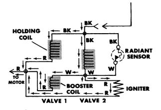
Because of the very low resistance of the hot igniter, most of the line voltage is dropped across the secondary coil. Only a small percentage is dropped across the booster coil and igniter.  The secondary coil now opens Valve
