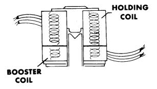
Both coils are needed to lift the armature and open the valve. The holding coil is strong enough to keep the valve open once the armature has been lifted. The second of the two valves is operated by the traditional one coil solenoid. This is called a secondary coil.
