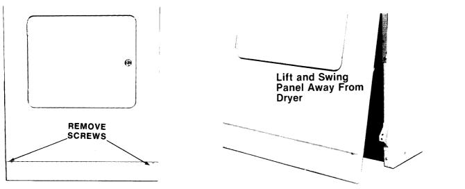
3. Front panel may be set off to one side or if necessary, the door switch wires may be disconnected and the front panel removed completely from the unit.
