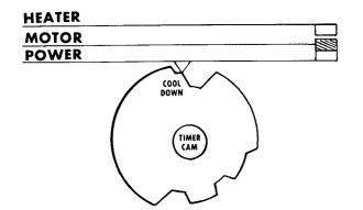
motor, the tumbler will continue to rotate and the air will continue to be pulled through the tumbler cooling the load before the dryer shuts off.
