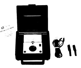
The Maytag appliance test meter is most effective when used to detect open or closed circuits in an electrical component. This method of testing is often referred to as "continuity testing" and is the easiest means of checking a part.
