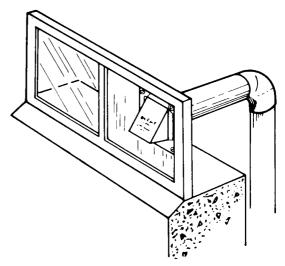
Install ductwork from the dryer to exhaust hood. All joints must be made so exhaust end of one pipe is inside the intake end of next pipe. On flexible metal ductwork, all joints should be secured with a 3-4630 clamp. **DO NOT** use sheet metal screws when assembling rigid ducting. These should be taped.
