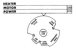
As the timer advances to the off position, the switch arm drops into step one. This breaks the circuit to the heater. Since the circuit is still made to the drive
