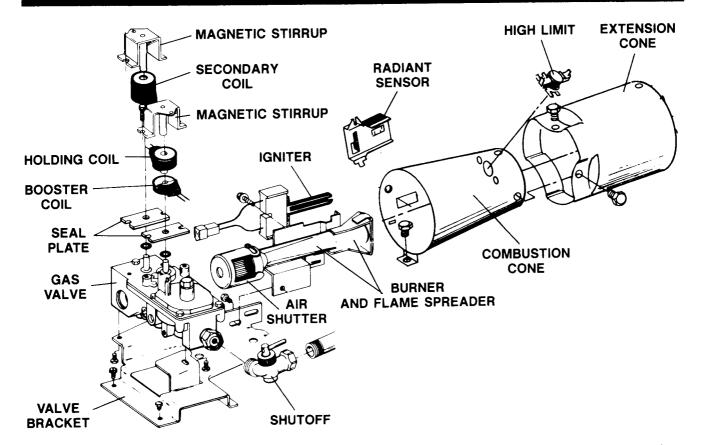
The gas controls utilize a direct ignition system (there is no pilot light). The three major components of the gas are: Igniter, Radiant Sensor and Gas Valve.
