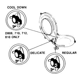
The cool down thermostat is only used on electronic control dryers. It is possible that you may encounter one or two regulating thermostats. Any dryer with one regulating thermostat, the thermostat will be a delicate temperature thermostat.
