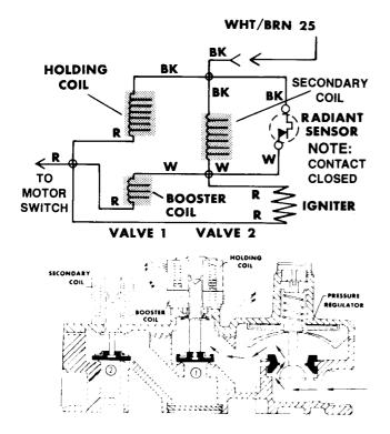
First, note on the wiring diagram that the radiant sensor contacts are wired across the secondary coil. This effectively bypasses current around the secondary coil when the radiant sensor contacts are closed. Valve 2 cannot open with the radiant sensor contacts closed.
