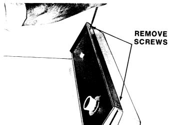
Tip control panel assembly forward. NOTE: When reinstalling, engage tabs on backup plate in slots of console.
