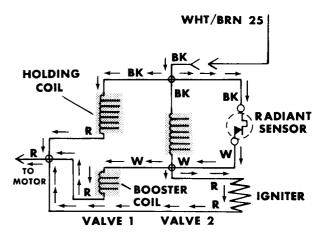
Because the secondary coil on Valve 2 is bypassed by the radiant sensor contacts, Valve 2 remains closed and prevents the release of gas.
