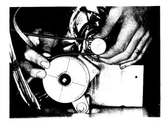
6. With the right hand, position the belt over the top of the idler pulley and begin to work it around the circumference of the idler pulley while pushing the pulley up and to the left.
