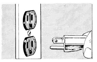
If a mating wall receptacle is not available. Contact a qualified electrician to have the wall receptacle replaced. If there is any question, local building officials or electrical utility should also be consulted.
