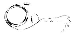
The motor test cord may be used to electrically check operation of the drive motor while still installed in the unit. Testing of the motor in this manner determines whether or not it will run independently of other electrical components.
