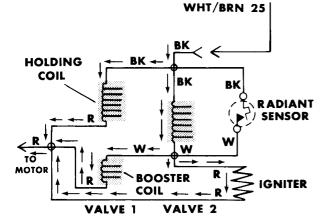
Because of the very low resistance of the hot igniter, most of the line voltage is dropped across the secondary coil. Only a small percentage is dropped across the booster coil and igniter.
