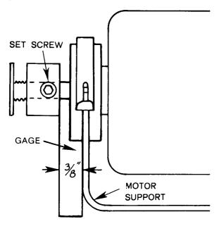
When replacing the motor pulley make sure the set screw aligns with the flat side of the motor shaft. Tighten set screw securely.
