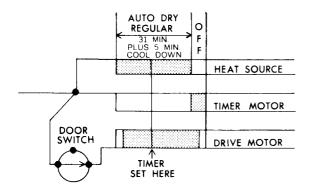
With the timer set in this position, the circuits are completed to the heat source and drive motor. NOTE: The switch controlling the timer motor is open.
