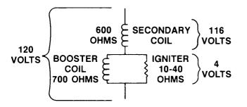
2. The secondary coil now opens Valve 2 releasing gas across the still extremely hot igniter. The burner flame is ignited.
