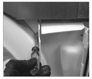
6. Force the plastic flange of the housing to the right and remove Drum
