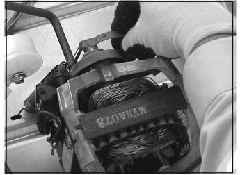
11. Rotate motor counterclockwise approx. 45 degrees. Lift up on the back of the Motor and pull out of the Front Support.
