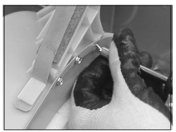
8. Carefully work Blower Wheel off the Motor Shaft.
