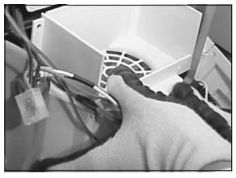
7. Loosen screws on mounting plate and remove Blower Assembly.
