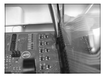
4. Slide the entire Logic Board to the left, to allow the white tabs to align with the elongated slots.
