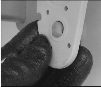
4. Remove center hanger, and remove assembly.
