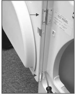
Door Hook Removal1. Rotate hooks 1/4 turn counterclockwise to remove
