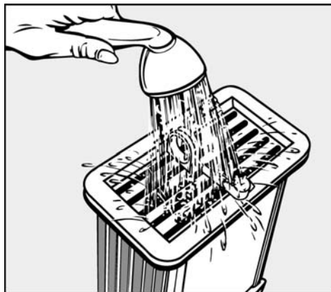
Figure 055-9: Rinsing the Condenser Box from the front.
