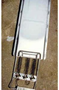
On Whirlpool the heating element slides into a long sheet metal box which is clamped onto the rear of the dryer. The bracket that holds the heater box is held in by one screw. The small bracket squeezes the heating element chamber up against the back of the rear basket frame. It is accessible in two ways.
