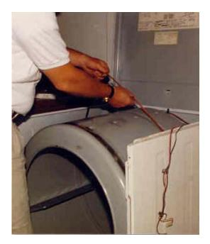
The current style Norge has not been on the market long enough to develop a pattern of failures, except for one thing. The heating element has problems. On the side of the heating element is a thermal fuse. When the thermal blows, just like it does on the Whirlpool design, the dryer goes dead. The thermal fuse is mounted right next to the high limit thermostat. Apparently there is a design problem and the heat builds up too easily. It also appears to be very sensitive to partial vent clogging.
