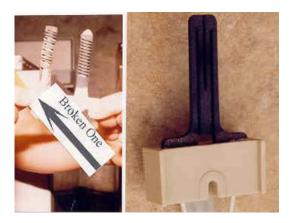
Diagnosing and Repair of Carbide Igniter Systems
