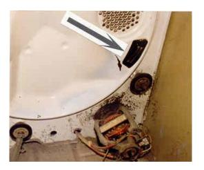
These systems work well. If anything such as a melted crayon or dirt shorts the bars out, the dryer will read "wet" continuously and the dryer never shuts off. The problem is rarely the printed circuit board.
