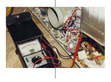
Fig042\_12 A Badly Burned Line Cord
