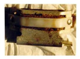
Fig043\_05a Worn Out Front Support
