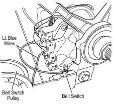
Figure 10. Checking the belt switch.
