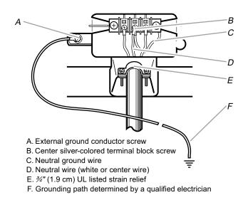
3. Connect the other wires to outer terminal block screws. Tighten screws.
