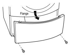
**Figure 14.** Pull the toe panel down to clear flange, then pull panel out.
