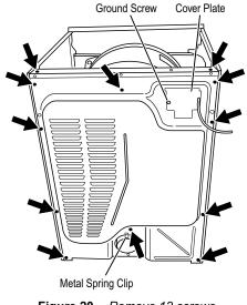
Figure 20. Remove 12 screws.
