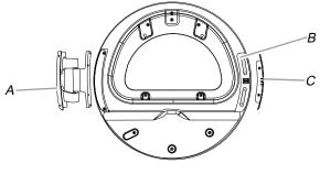
A. Door hinge B. Plug strips C. Hinge cover
