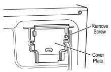
Figure 3. Remove the cover plate.
