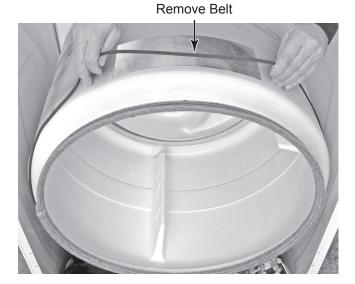
c) Lift the drum and remove it from the dryer cabinet.
