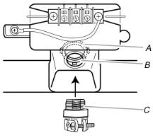
A. Removable conduit connector B. Hole below terminal block opening C. Strain relief threads  Put direct wire cable through the strain relief. The strain relief should have a tight fit with the dryer cabinet and be in a horizontal position. Tighten strain relief screw against the direct wire cable.
