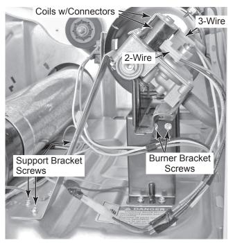
Remove the two screws from the coil retaining bracket.
