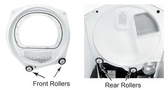
a) Pry the sides of the triangular ring out of the groove in the roller shaft with a small screwdriver.
