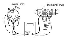
**Figure 4.** *Plug-to-terminal connections for electric dryer.*
