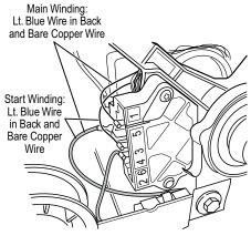
**Figure 9.** Main and start winding measure points.
