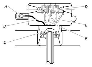
A. External ground conductor screw B. Ground wire (green or bare) of power supply cord
