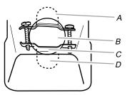
A. Strain relief tab pointing up B. Hole below terminal block opening C. Clamp section D. Strain relief tab pointing down • Put power supply cord through the strain relief. Be sure that the wire insulation on the power supply cord is inside the strain relief. The strain relief should have a tight fit with the dryer cabinet and be in a horizontal position. Do not further tighten strain relief screws at this point.
