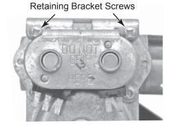
9. Lift the two coils off their cores and remove them.
