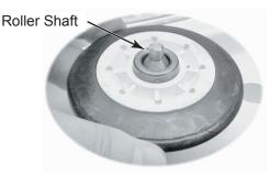
c) **To remove the roller shaft,** remove the 9/16<sup>"</sup> nut and washer from the roller support, and remove the support and remaining triangular ring.
