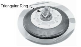
b) Slide the roller off the roller shaft.
