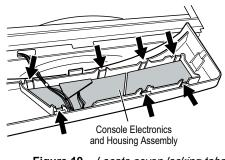
Figure 19. Locate seven locking tabs.
