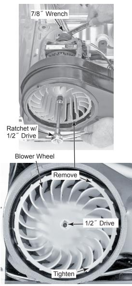
c) Remove the four screws from the blower housing and exhaust duct and remove the housing.
