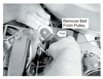
b) Slide the belt off the front of the drum and remove it.
