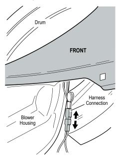
**Figure 12.** Disconnect sensor from wire harness.
