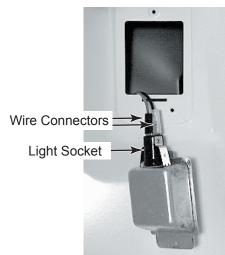
8. Squeeze the locking arms and remove the socket from the drum light holder.
