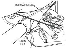
Figure 7. Carefully remove drum belt.
