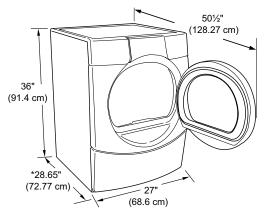
Most installations require a minimum 5<sup>"</sup> (12.7 cm) clearance behind the dryer for the exhaust vent with elbow. See "Venting Requirements."
