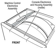
**Figure 15.** Locate the electronic <sup>T</sup> assemblies.
