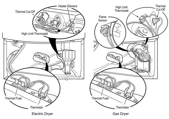
Figure 11. Thermal Components, viewed from front.
