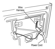
**Figure 5.** Power cord-to-wire harness connection for gas dryer.
