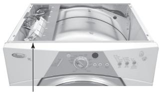
Machine Control Electronics Assembly
