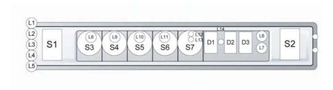
L - LED, S - Push-button, F - Fault code on the display
