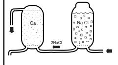
0,05 - 0,23 litres of water flow into the salt container, where the Ca is replaced by Na. CaCl<sub>2</sub> is flushed into the machine.
