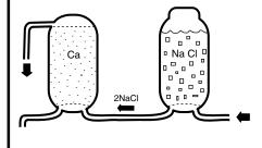
0,05 - 0,23 litres of water flow into the salt container, where the Ca is replaced by Na. CaCl<sub>2</sub> is flushed into the machine.
