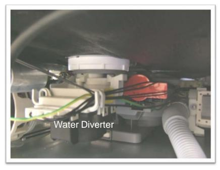
Circulation motor/pump is removed in the same manor as the 3,000 series, however there is less room to maneuver due to the taller tank. It may be easier to remove and replace the motor/pump as a complete assembly.
