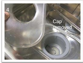
Remove strainer: With cap removed from sump there is access to the impellor of the drain pump for clean out
