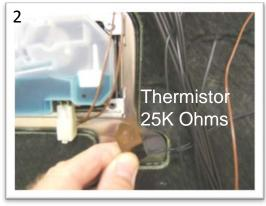
Remove thermistor from right side of lower clamp (3,000 series only)
