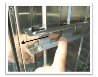
Slide out the ball bearing plastic holder which should contain 4 bearings. Check the bottom of the tank for broken off plastic pieces or ball bearings which may have fallen out.
