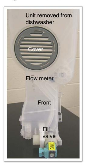
The air break contains the fill valve and the flow meter, it is fastened to the side of the tank with the cover (from the inside of the tank) and a single screw on the outside.
