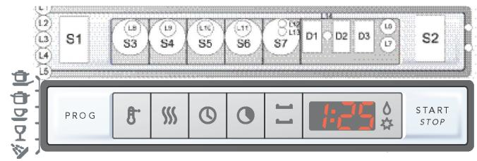
When the main power switch is turned on after replacing the control unit, the variant setting menu is displayed.
