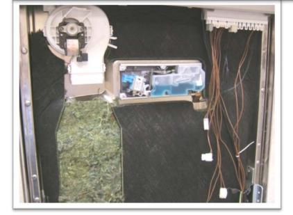
If wiring from a component to the control board or from the control board to a component, check with the wiring diagram for correct location of connectors.
