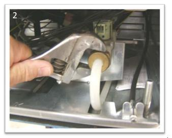
Unscrew supply hose fitting (turn off water first)
