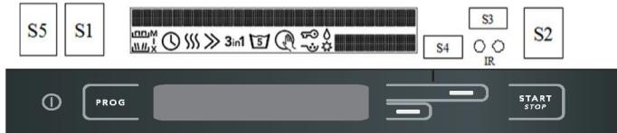
Turn off the main power switch, wait at least 5 seconds. Press and hold the Program and Start buttons then turn on the main power switch. Release the Program and Start buttons.
