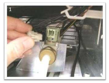
Remove the Molex connector from valve
