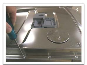
Remove the screws down each side
