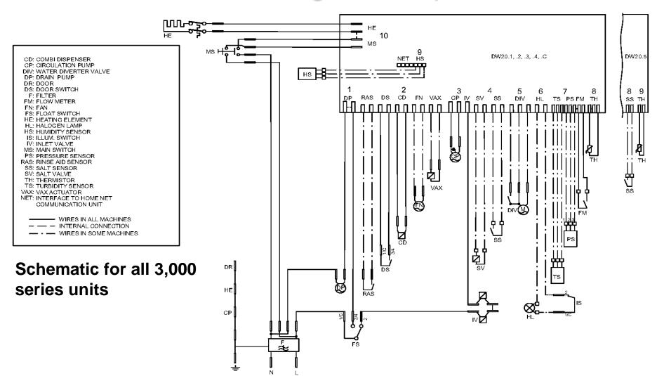
Dispenser 300 Ohms: Circulation pump 22 Ohms: Water diverter valve 2600 Ohms: Filter 1 mega Ohm: Heating element 12 Ohms: Fill valve 950 Ohms: Thermistor 25,000 Ohms: Wax actuator 1100 Ohms: Fan motor 180 Ohms: Drain pump 25 Ohms
