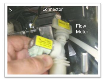
Remove connector from flow meter
