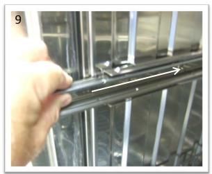
Slide the newly assembled bearing holder into the track, then slide the rack rail into the bearing holder. Finish off by reinstalling the rear rail stop.
