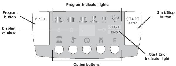
**Water intake adjusting** (after week 16, 2005) Press the program button until "1" appears in the display. Press the program button and index through the following: Display shows **0**: Normal water intake, **1**: increase 5%, **2**: increase 10%, **3**: increase 15%, **4**: Time controlled water intake, **5**: Increase 5% on time control, **6**: Increase 10% on time control, **7**: 15% increase on time control. Confirm choice by pressing start. The program returns to the main menu.
