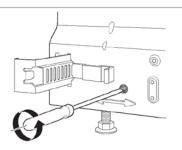
Check that there is a 1/8 inch (3mm) space between the top of the dishwasher door and the underside of the counter.
