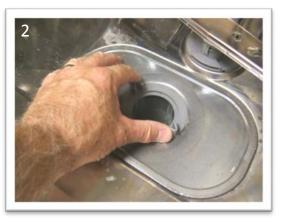
Rotate fine mesh filter counter clockwise.
