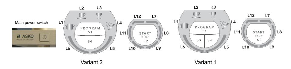
If the control is replaced the machine will automatically be in the variant setting menu when the power is turned on. Press the program button repeatedly, the display will alternate between pan symbol (L1) flashing, (variant 1) and the shower symbol (L4) flashing, (variant 2). Choose the variant, then confirm this selection by pressing the start/stop button. The program will then revert automatically to the main menu.
