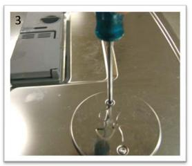
To remove assembly, disconnect Molex connector from wax motor and fan motor. From inside the door remove the two screws holding stainless assembly cover. Grasp the inner black cover and twist counterclockwise. Remove unit from door.
