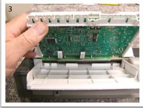
After removing the wire connections and removing control panel from the unit, lay it down on a protected flat surface. Not all control boards can be removed from the panel intact, for example the FI unit shown above. In this case separate the casing by using a flat blade screwdriver and prying the tabs apart see (2)
