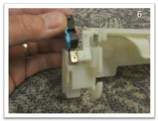
To remove door micro switch, bend tab on switch assembly and slide switch up and out of the housing.
