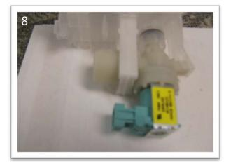
Snap clamp into housing to lock in place
