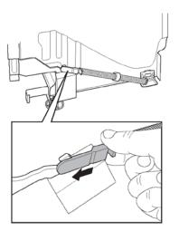
If you want to make small adjustments to the spring, hold the back end with one hand and turn the forward mount clockwise or coun terclockwise one or more times. Turn the mount clockwise to increase spring tension and counterclockwise to reduce spring ten
