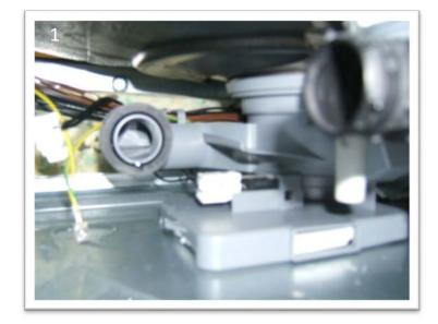
The float switch is mounted in the sump housing. In the event of water overflowing into the base pan, a Styrofoam float rises up and activates a micro switch turning on the drain pump.
