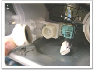
Disconnect pex hose and Molex connector from valve
