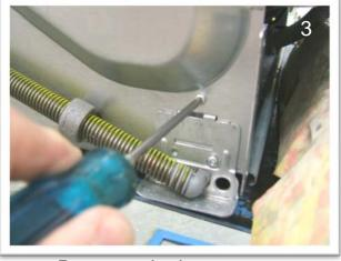
With a straight blade screwdriver rotate cover counter clockwise to remove. Remove single screw on outside and two from the inside of the tank.
