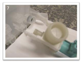
Push the spigot of valve into housing making sure the seal is in place
