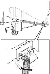
5. Replace the back end of the spring by holding the spring at a right angle to the side of the dishwasher and pushing the end of the spring into the hole, then turning the spring in toward the dishwasher.
