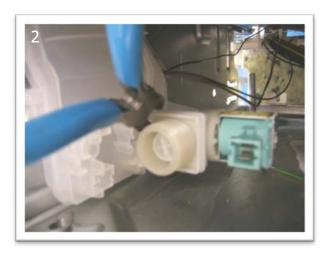
Cut through retaining clamp with cutters
