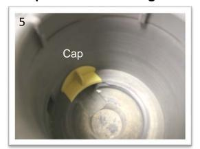
Sump drain cap sits down in the sump area inside the outlet to the drain pump
