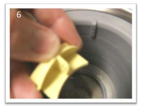
This cap must be in place in order for the machine to drain correctly
