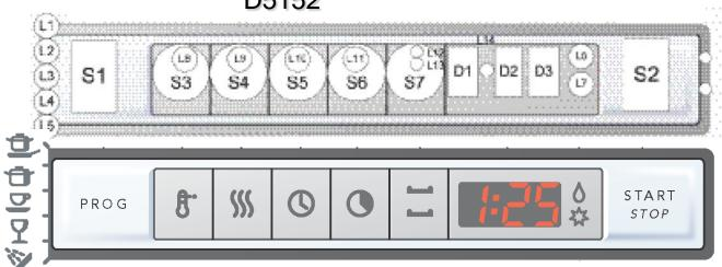
Turn off the **main power switch**, wait at least 5 seconds. Press and hold the **Program** and **Start** buttons. Turn on the **main power switch**, wait until the LEDs have lit, release the **Program** and **Start** buttons. The most recent fault code if there is one will be shown in display **D2** AND **D3**. Press the Program button to activate the component test. These are activated in order after each button press and are shown in D3.
