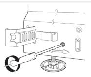
Place the spirit level on the dishwasher door to check that the machine is level and adjust if necessary. The door must be fully closed!
