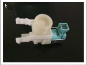
Attach the clamp to the valve as shown
