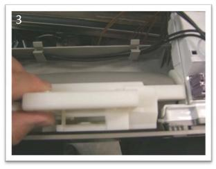
After removing the outer door remove the 2 screws on top of the inner door. Ease the control panel from the tabs in the top of the inner door. Release wiring to door switch and lift latch from cradle.
