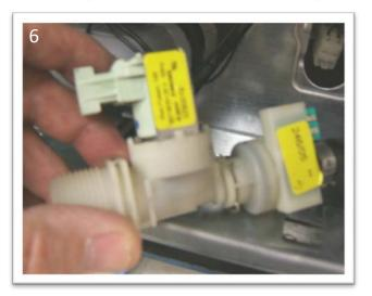
Fill valve is connected to flow meter with a push/turn bayonet type fitting
