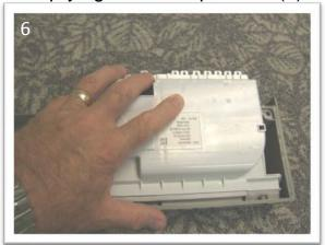
The new control board will install into the control panel as a complete assembly. Insert the touch pad end into the control panel first then snap the unit into place.
