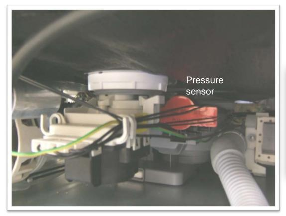
Sensor is a push fit into housing and is held with a tab fitting
