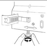
Screw in the back foot completely by turning the adjustment screw at the front counterclockwise. Use a flat-bladed or a 1/4 inch nut driver.
