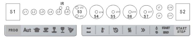
Turn off the main power switch. Wait at least 5 seconds. Press and hold the program and start buttons, turn on the main switch, wait for the teardrop symbol to light on the right side of control, release the program and start buttons. **L10** AND **L11** flash.
