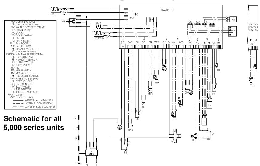
Dispenser 300 Ohms: Circulation pump 32 Ohms: Water diverter valve 2600 Ohms: Filter 1 mega Ohm: Heating element 12 Ohms: Fill valve 950 Ohms: Thermistor 60,000 Ohms: Wax actuator 1100 Ohms: Fan motor 180 Ohms: Drain pump 25 Ohms.
