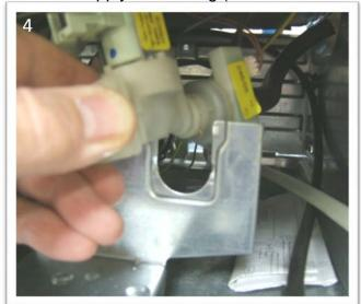
Slide the valve out of the bracket
