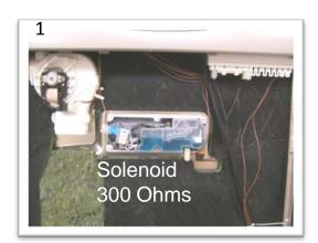
Detergent & rinse aid dispensers are combined into one assembly & is fastened to the inner door with 2 clamps
