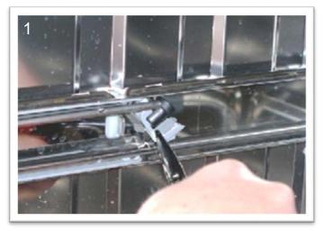
To remove ball bearing holder for upper rack rail, use a flat blade screwdriver or needle nose pliers and remove the rear rail stop by easing the bottom of the stop out of the notch in the rail. Now slide the rail out of the track.
