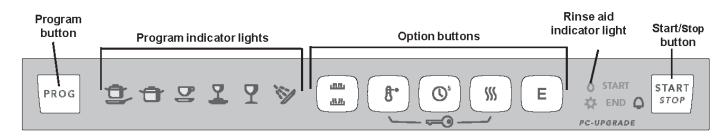
Turn off the main switch, wait for at least 5 seconds. Keep the program and start buttons depressed and turn on the main switch, release the program and start buttons. The most recent fault will be indicated as L1 - L6.
