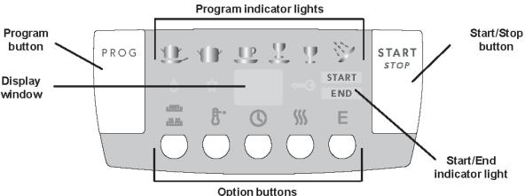
Turn off the main switch, wait for at least 5 seconds. Keep the program and start buttons depressed and turn on the main switch, release the program and start buttons **at once**. The display lights up after 5 seconds. The most recent fault will appear in the display F1, F2, etc.
