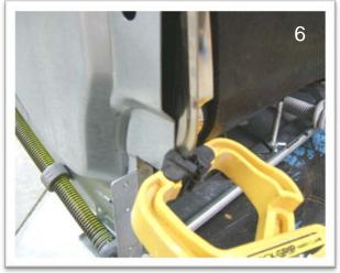
Block side wall away from tank, and slide the air break out from its location. When reinstalling make sure the seal is in place and use a clamp to pull side support to tank so that screws will engage.
