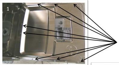
Open the dishwasher door, there are 2 screws at the bottom of the inner door and 3 down each side. 5 or 6 if the unit is an FI model
