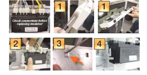
▲ <u>CAUTION</u> – 75% of all controls returned for analysis check out OK. Most control issues are due to loose connections.
