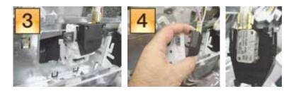
**<u>HINT</u>**: Make sure plastic latch tabs are aligned & metal console tabs are bent back completely during reassembly.
