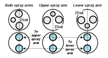
Water switches are used to divert water to upper or lower spray arms. Separate actuators aren't needed.
