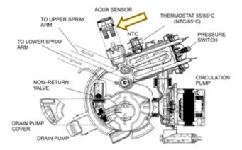
Dishwashers still operate adequately if aqua sensors fail. Customers will only notice aqua sensors failing if they see their dishwashers running slightly longer or their electric and water usage getting slightly higher.
