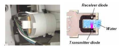
If water is clean enough, it will be kept for the wash cycle. If not, the aqua sensor directs the dishwasher to add an additional pre-rinse or pre-wash cycle.
