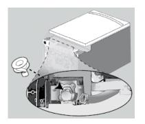
Attach the hot water line to the 90° elbow and route it underneath the unit toward the hot water connection. Make sure the line doesn't contact any moving parts.
