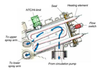
Filtered water from the sump flows through the circulation pump into the flowthrough heater. All heaters are protected by a 185°F Hi-limit (high temperature cutout) and by a flow switch which prevents heaters from operating when no water is flowing.
