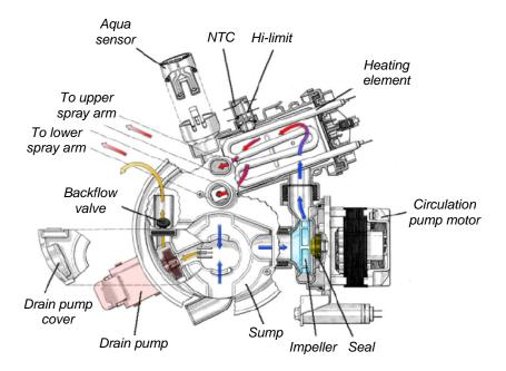
The aqua sensor, drain pump, NTC, Hi-limit and backflow valve are near the heater under the sump. The aqua sensor senses water cleanliness – dishwashers add or subtract rinses as needed. The NTC senses water temperature. The Hi-limit shuts off the heater if the water gets too hot. The backflow valve prevents waste water from entering the dishwasher.
