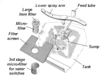
The sump holds the drain pump cover and check valve.
