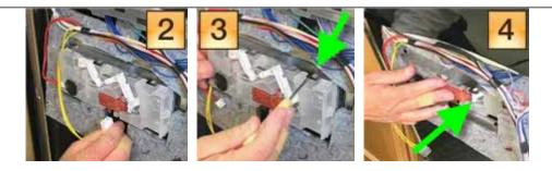
**<u>CAUTION</u>**: Inner door edges are sharp! Cover door edges and remove dispenser carefully.
