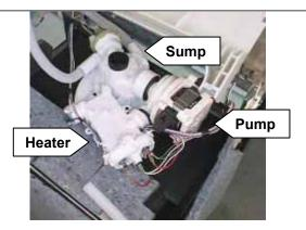
Access to circulation pump, heater and sump after base has been removed.
