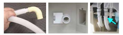
To remove the internal drain hose, remove a white plastic hose lock and pull the hose from the water level control.
