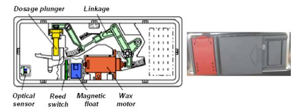
The white plastic linkage opens the detergent dispenser door, then cocks in place to dispense rinse-aid when the wax motor operates again. After the 2nd operation, the linkage resets for the next wash.
