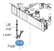
If there's water in the base or the float switch isn't working, error code **E5** is possible.
