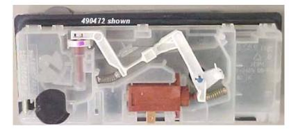
During each wash program, the wax motor opens twice, once to dispense detergent and again to dispense rinse-aid. The wax motor opens the same -- linkages open the detergent door & operate the rinse-aid dosage plunger. Dispensers can have reed switches or optical rinse-aid sensors.
