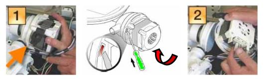
**<u>CAUTION</u>**: Don't grab motor next to the capacitor to avoid jamming your hand on the capacitor.
