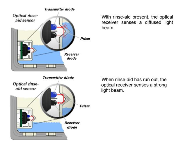
When rinse-aid has run out, the optical receiver senses a strong light beam.
