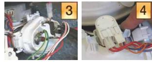
5. To remove flow switch, carefully pry housing away from switch (until tabs clear switch), then snap switch out. Note flow switch can be removed from right side without flipping dishwasher upside-down.
