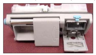
**<u>HINT</u>**: Resistances of actuator and rinseaid sensor cannot be measured.
