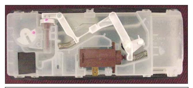
**NOTE**: The white plastic linkage 1st opens the detergent dispenser door, then cocks in place to dispense rinse-aid when the wax motor operates the 2nd time. After the 2nd operation, the linkage resets itself so it will open the dispenser detergent door for the next wash program.
