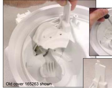
Drain pump covers were changed from **165263** to **423419** to provide better water flow and resistance to jamming.
