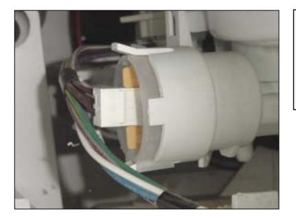
**NOTE:** If water is clean enough, it will be kept for the wash cycle. If not, the aqua sensor directs the dishwasher to add an additional pre-rinse or prewash cycle.
