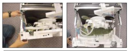
Carefully pull base away from tank & sump
