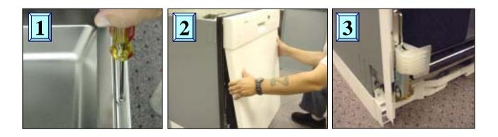
**<u>HINT</u>**: The fascia panel and door don't need to be removed to access the circulation pump. However, they must be removed to completely remove the tank.
