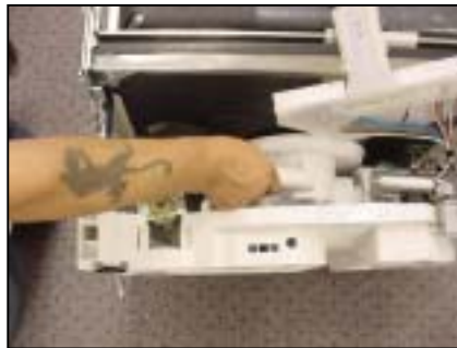
Pull out sump inlet hose
