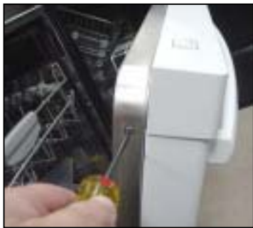
Removing door screws
