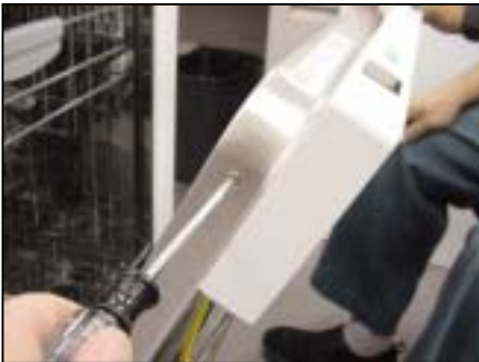
Remove panel screws
