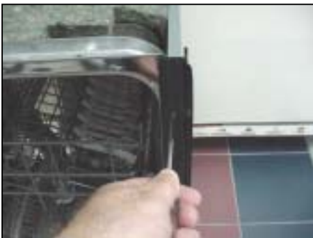
Remove panel screws
