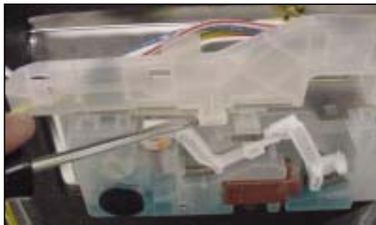
Disconnecting wire harness
