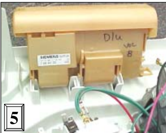
Sliding module out
