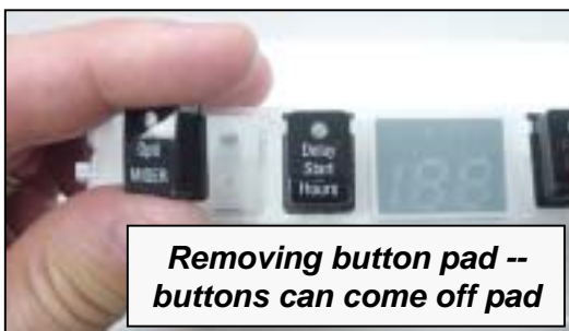
Align tabs when reassembling
