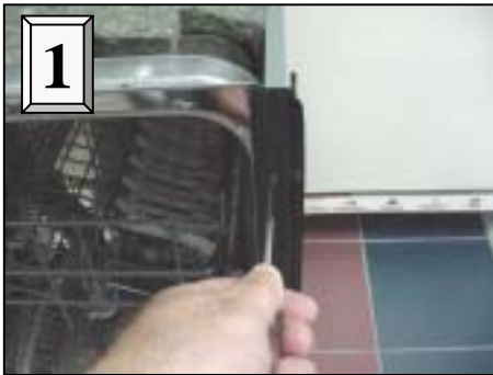
Removing trim strip screws
