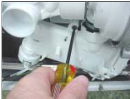
Remove heater screws
