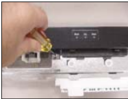
Removing fascia screws
