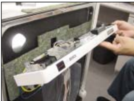
Replace fascia panel
