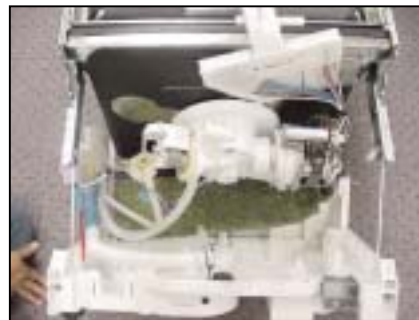
Carefully pull base away from tank & sump
