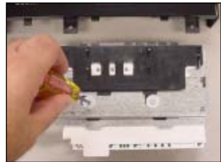
Removing module screws
