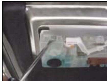
Bending retainer tabs
