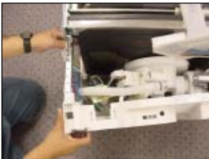
Carefully pull base away from tank & sump
