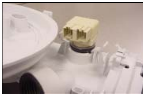
Remove cover & pull tabs
