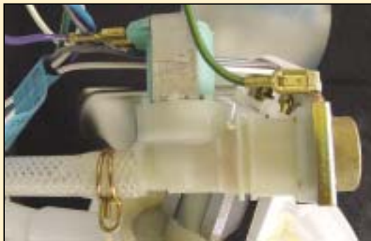
Removing hose clamp
