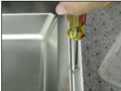
Remove inner door screws
