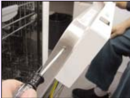
Removing door screws
