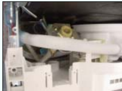
Disconnect water valve from base
