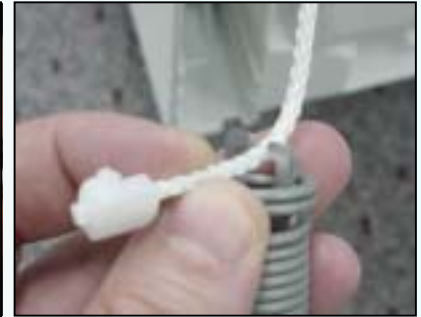
Pull out door springs from base & disconnect cords
