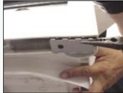
Pull out door springs from base & disconnect cords
