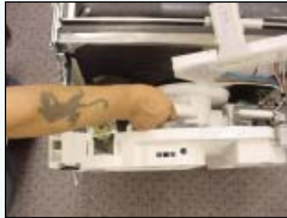
Pull out sump inlet hose
