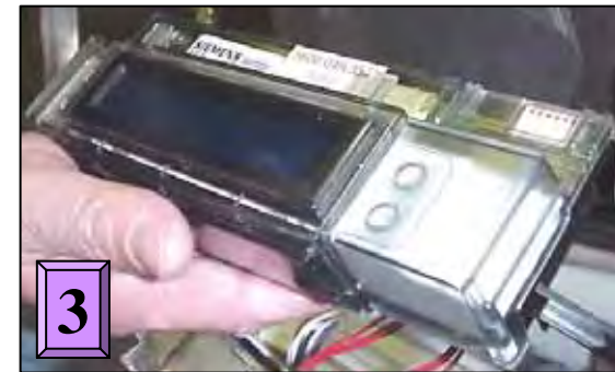
Removing display module
