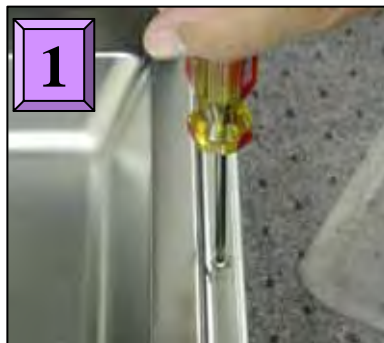
Removing door & fascia
