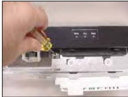
Removing fascia screws
