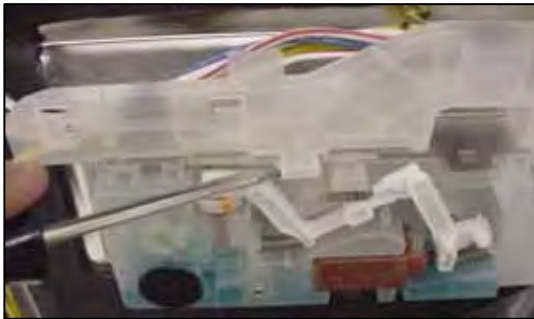
Disconnecting wire harness
