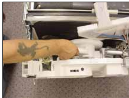
Pulling out sump hose
