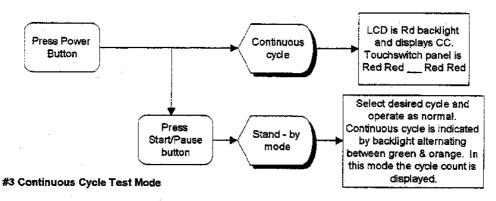
Once a mode has been entered, press Power to exit diagnostics except Display and Show Off modes) which require the plug to be removed from the power socket.
