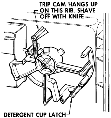
Figure 10 - GSD2500 Detergent Cup Latch
