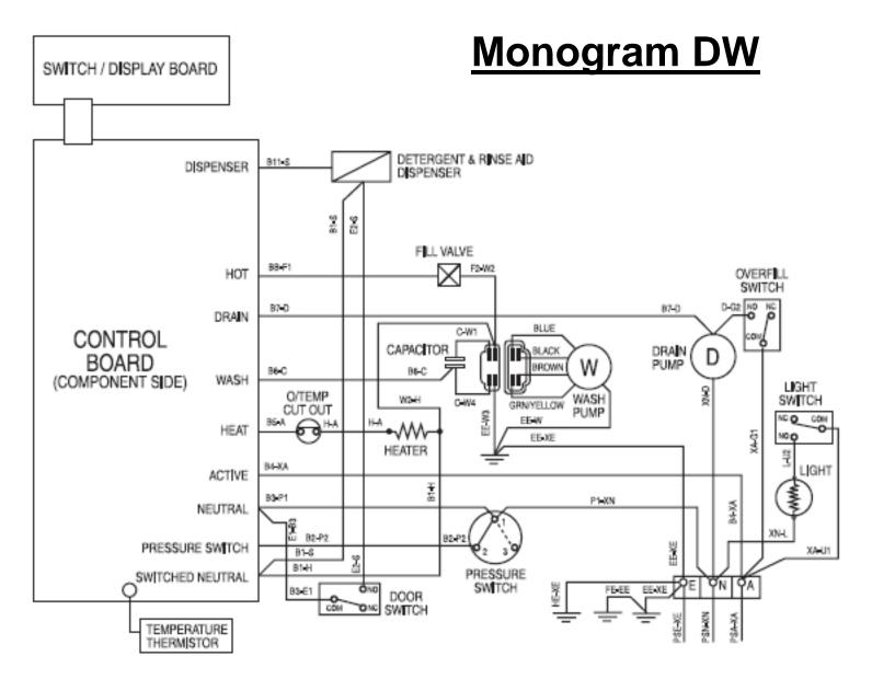
NOTE: Schematics and Wiring Diagrams label L1 as A for Active, N for Neutral, and Ground (GND) as E for Earth.
