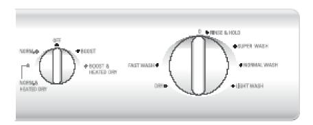
The Monogram 5600 model is fitted with a soft-set rotary self-indexing timer, which has a detent mechanism to index the timer control knob to the 'start' position of a wash program. Six detent positions from the 12 o'clock position form the actual programs as follows: Rinse & Hold, Super Wash, Normal Wash, Light Wash, Dry and Fast Wash.
