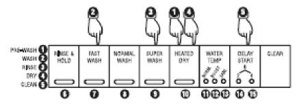
4.2.1.3 To cancel the display, repeat the sequence above : Heated Dry, Fast Wash, Super Wash, Heated Dry, & Delay Start with the door closed.
