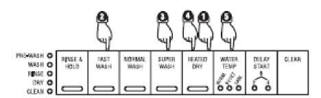
4.2.4.2 The fault codes (if any are recorded), will then be displayed by flashing the relevant program/option LED's. Pressing the Clear button will clear the retained fault codes from the memory and the power board control (PCB) will be in standby mode with all LED's OFF.
