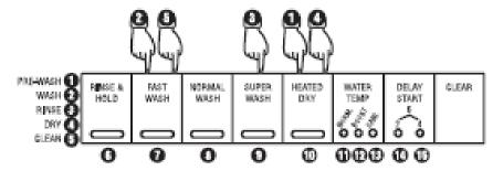
4.2.2.3 To cancel, either enter the RELAY/TRIAC OUTPUT TEST (refer to next section 4.2.3) or follow the sequence: Heated Dry, Fast Wash, Super Wash, Heated Dry and Clear with the door closed.
