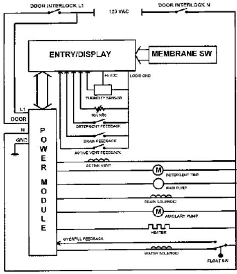
NOTE: Junction box L1 & N are not shown. (They feed transformer on power module through P1.)
