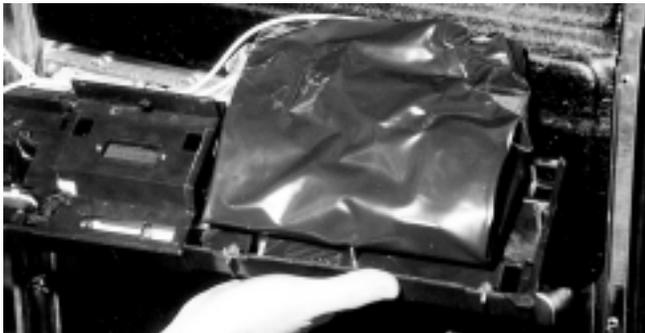
Sealed PVC Drip Sheet covers the Power Control Board.
