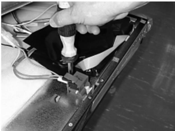
**5.2.44.2** Remove both 1/4" terminals and wires from the Microswitch. Pry open the clip holding the Microswitch in the Latch Housing with a small screwdriver, then remove the Microswitch.
