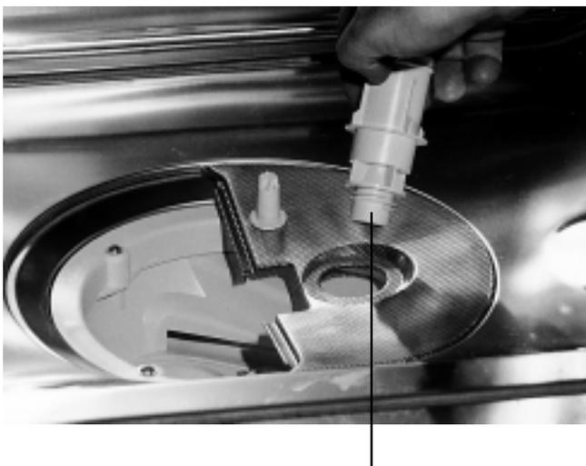
Unscrew Lower Spray Arm Support to remove
