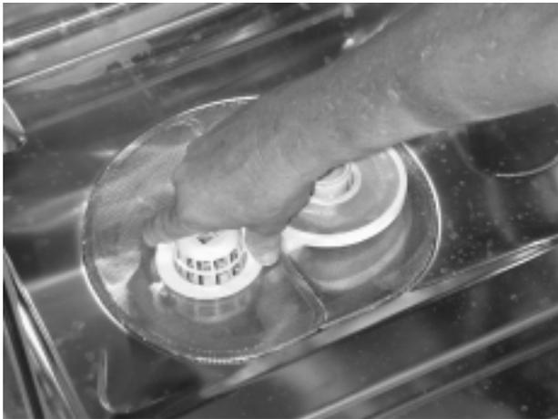
Rotate counter clockwise and lift up to remove.
