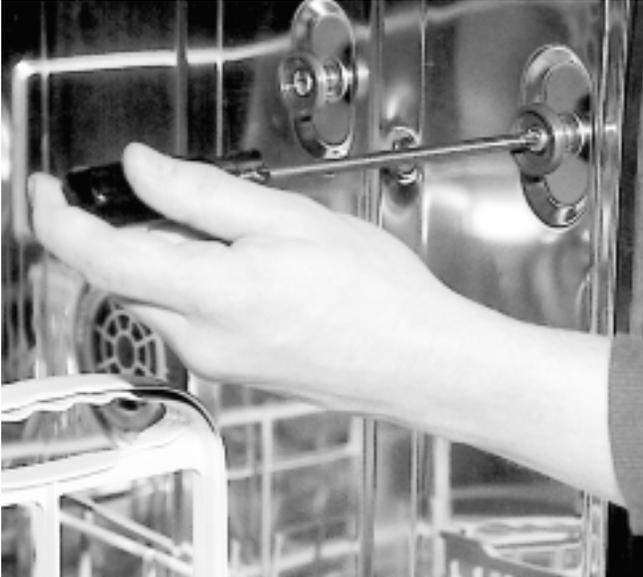
5.2.17.6 Ensure the stainless steel cup washer, which houses the rubber "O" ring, is identified with the recess side of the washer to the surface of the stainless steel tub.
