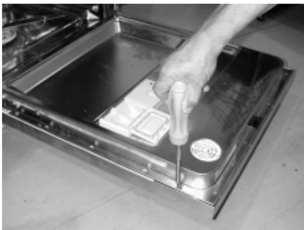
Remove the 6 screws side and top of door
