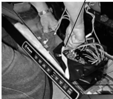
3 screws and 2 clips in door panel plastic housing
