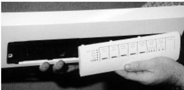
**5.2.7.4 Carrier Panel:** The Carrier Panel is removed from the assembly by bending the two side metal retainers on the Control Panel to a vertical position.
