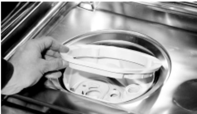
5.2.36.5 Remove Sump from beneath the stainless steel tub.
