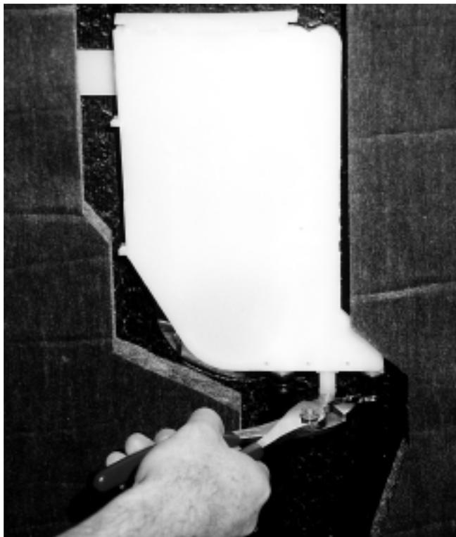
**5.2.19.2** Grasp the hose and turn and remove from the Siphon Break spigot.
