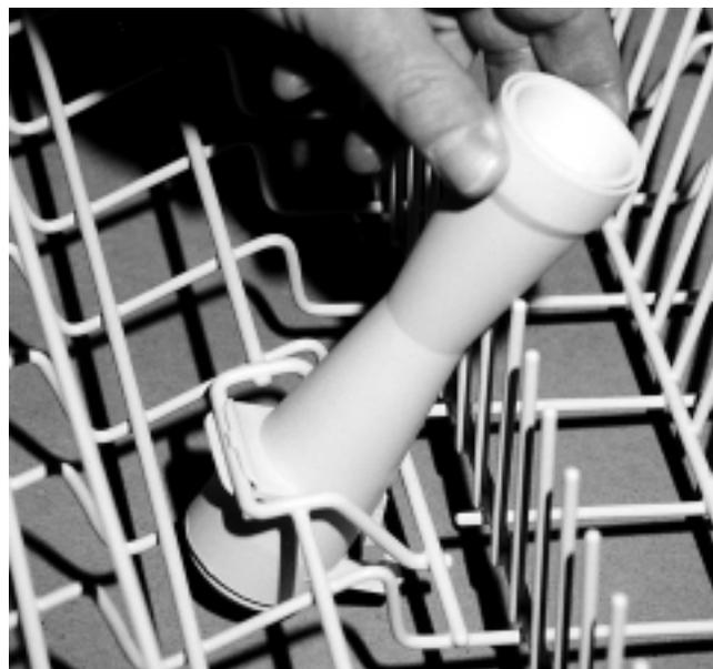
**5.2.13.4** Prize the Upper Venturi Assembly from the cross bar and remove the Upper Venturi Assembly from the underside of the Upper Basket.
