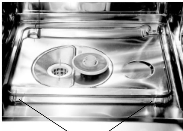
Two front Element retaining brackets.
