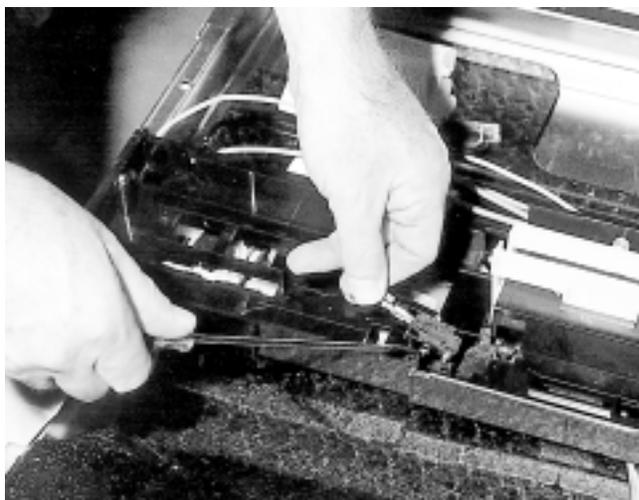
**5.2.43.3** Repeat procedure with lower retainer clip, although clip will require to be unlatched without the aid of a mounting hole to gain purchase. Carefully lift Microswitch from the two mounting posts and lift clear. Reassemble the dishwasher in reverse order. To reinstall the Microswitch a replacement cable tie is required.
