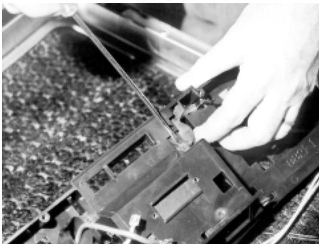
**5.2.45.3** Twist the Microswitch Lever and remove from the front central square aperture of the Control Panel Carrier Frame.
