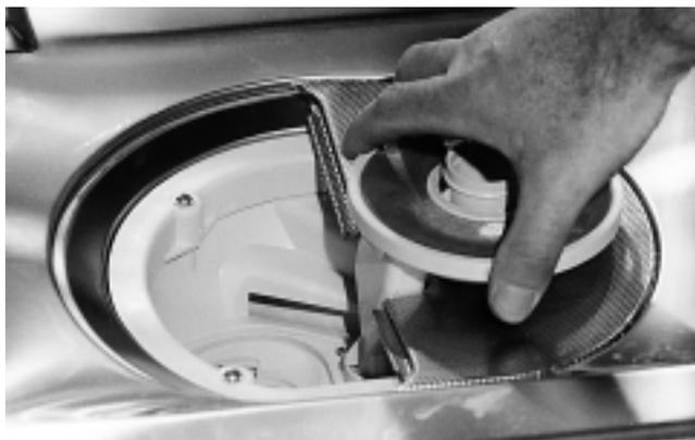
Recuperative By-Pass Filter - Pull Filter up to remove
