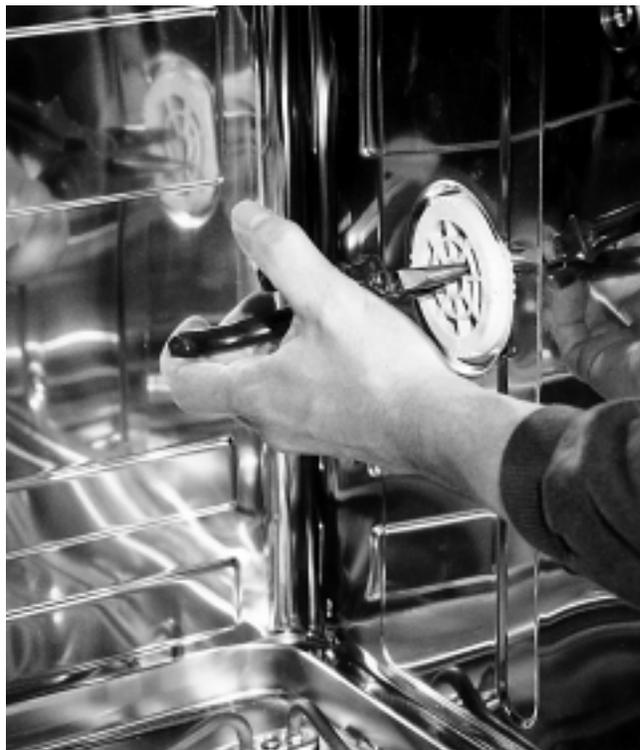
Remove Siphon Break Nut with pointed nose pliers.
