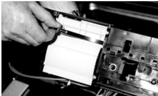
**5.2.41.4** Grasp Door Handle on one end and lift outward to unclip spigot from Control Panel Carrier Frame.
