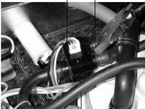
Wash Pump to Bypass Filter Hose
