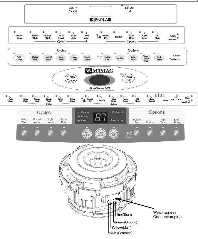
1/3HP 120V/60hz, 3.2 amps, 3250 RPM
