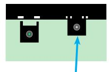
Keeper feet are inserted into small rectangular holes in the console, and screwed down
