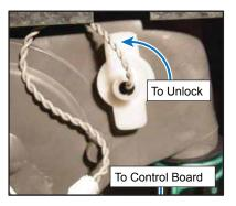
The image below shows the temp sensor in the unlocked position.
