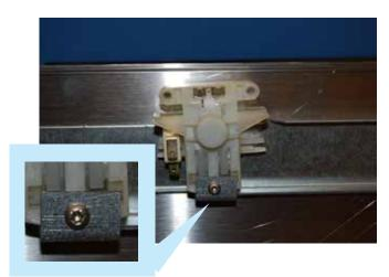
If door latch has been removed the following procedure should be used to install it for proper alignment.
