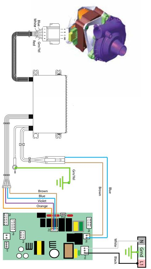
VDB541 Motor Control Circuits
