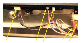
Remove wires going to the door latch and the three connectors going to the control pad and one connector going to start switch, shown above.
