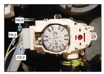
Disconnect the hose clamp connection from the diverter inlet as shown.
