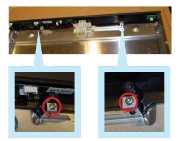
Remove the two T20 Torx screws, circled in red above to remove control assy from outer door panel.
