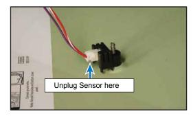
Note: Place base pan in a secured area. Take care not to damage the sensor.
