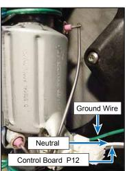
terminal on the heater housing. This image shows the connections.
