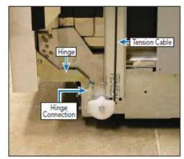
Remove C-Clip securing hinge.
