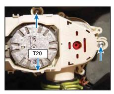
Remove the diverter from the sump assembly. The image below (left) shows the rear of the diverter and below right shows the sump area with the diverter removed.
