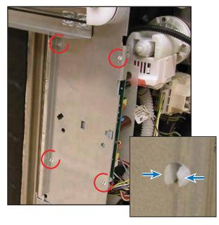
Disconnect P4/P9 wiring harness. Now carefully pull the board down and release from front.
