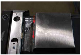
At this time the vent assembly can be removed from unit by lifting up and out,t from the top of unit.
