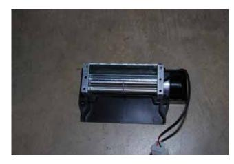
The blower can be released from mount by using a small screwdriver to release tabs, see inset in photo below. Release tabs and slide blower assembly and pull out of mount.
