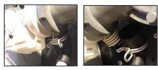
Next, release the drain motor from the sump assembly. Locate the release tab (indicated by the yellow dotted line, below left). Using a flat blade screwdriver, bend the tap in the direction shown by the arrow (below right) to release the pump from the main housing. Grasp the pump and rotate clockwise and the pump can be removed.
