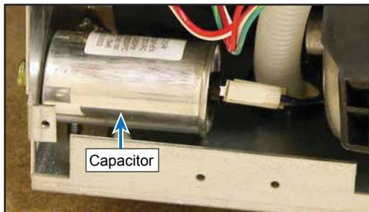
To test the capacitor, place the volt ohmmeter to the 1K  $\Omega$  ohm scale. Place the meter leads across the terminals of the capacitor and take a reading. Then reverse the meter leads on the capacitor terminals. A reading should be seen momentarily in one direction and an open circuit detected in the other. If this occurs the capacitor is good. The readings can also be made at the blue and yellow wire connection at the circulation motor
