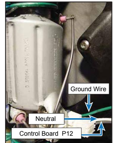
Next, disconnect the two clamps that hold the heater assembly to both the sump outlet (Arrow 1) and circulation pump inlet (Arrow 2) shown here. The heater can now be removed for service. You will need to transfer the two 1-1/2" OD hoses to the new heater assembly. The element is a 120-volt, 12 ohm, 10 amp, 1200 watt draw. It is controlled from P12 (gray) to Neutral on the main terminal block.
