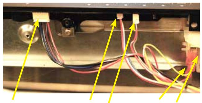
Remove wires going to the door latch and the three connectors going to the control pad as shown above.
