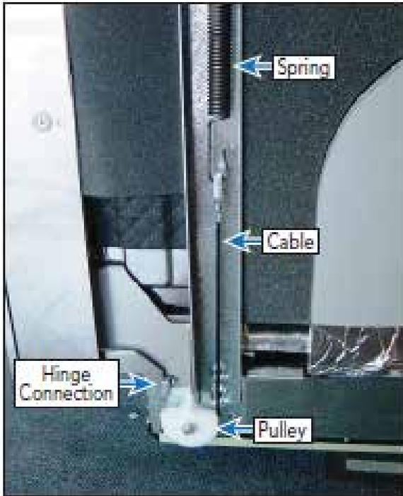
Below is a close-up view of the cable wrapped around the pulley. As the door opens or closes, the cable will ride along the roller creating a smooth movement in the door operation.
