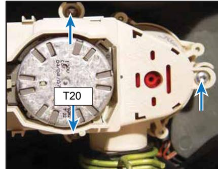
Remove the diverter from the sump assembly. The image below (left) shows the rear of the diverter and below right shows the sump area with the diverter removed.
