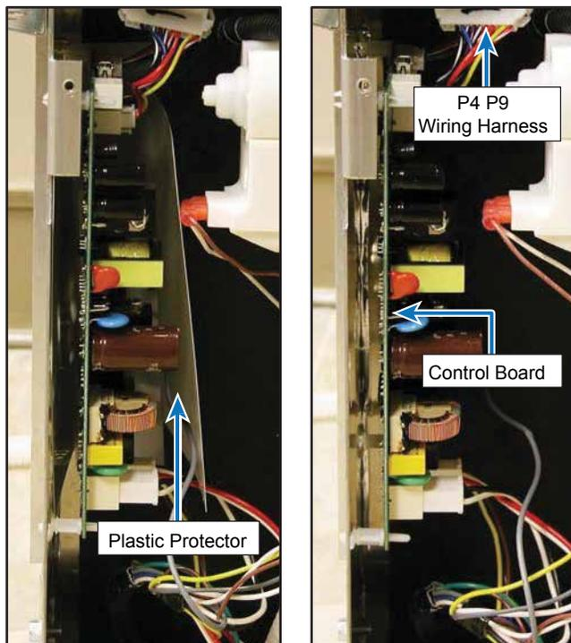
Disconnect P4/P9 wiring harness. Now carefully pull the board down and release from front.
