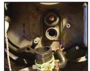
Disconnect the hose clamp connection from the diverter inlet as shown.
