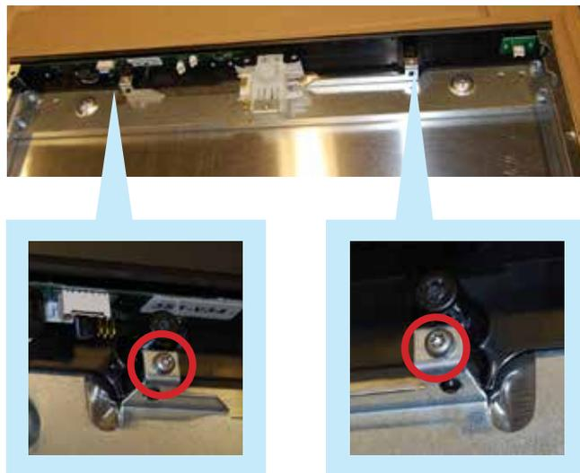
Remove the two T20 Torx screws, circled in red above to remove control assy from outer door panel.
