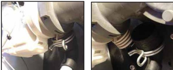
Next, release the drain motor from the sump assembly. Locate the release tab (indicated by the yellow dotted line, below left). Using a flat blade screwdriver, bend the tap in the direction shown by the arrow (below right) to release the pump from the main housing. Grasp the pump and rotate clockwise and the pump can be removed.
