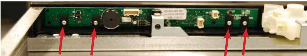
Remove the four T10 Torx screws as indicated by arrows in photo above, remove user interface board from control panel assembly.
