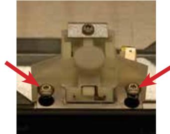
Remove the two upper screws at this time, they will be installed during the outer door panel assembly to the inner door assembly.
