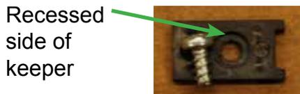
The plastic keepers have two feet on each keeper. These feet fit into matching slots on the control panel to ensure that User Interface Board doesn't move and is firmly anchored.
