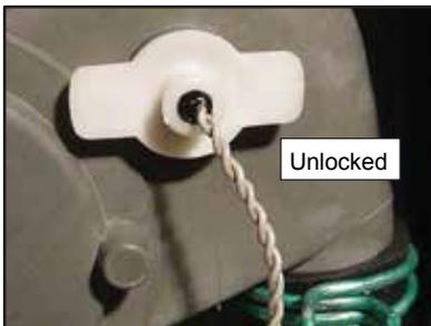
While grasping the tabs, pull the sensor out of the sump assembly as shown.
