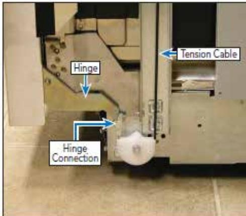
Remove C-Clip securing hinge.
