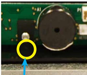
Keeper feet are inserted into small rectangular holes in the console.
