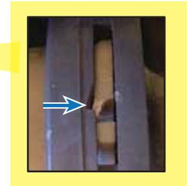
When reinstalling pump, make sure to bend the tab back in place to lock the pump in the sump housing.
