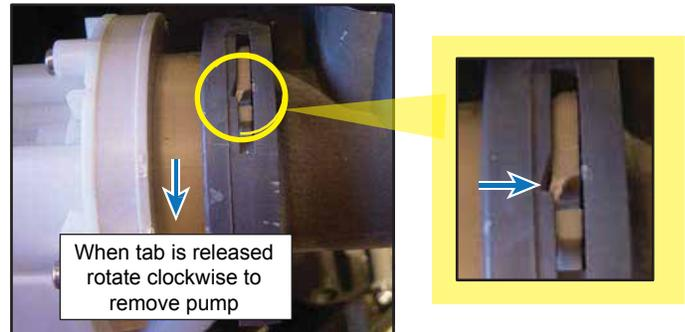
When reinstalling pump, make sure to bend the tab back in place to lock the pump in the sump housing.
