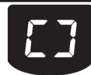
During Soil Sensing function (Interval 42), the LED display will show spinning "CLOCK" pattern. Clock countdown will begin once the cycle variation has been determined.
