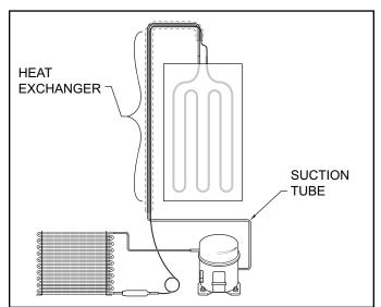
Figure 4-6. Suction Line & Heat Exchanger
