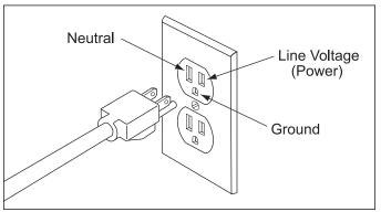
Figure 2-2. Power Cord and Wall Outlet
