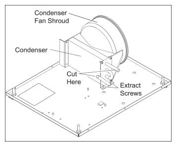
Figure 5-17. Condenser Removal
