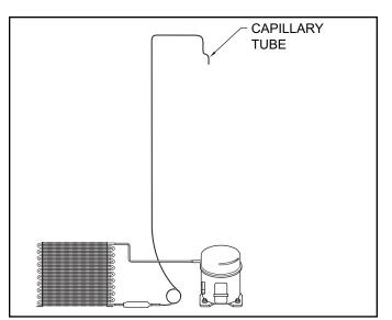
Figure 4-4. Capillary Tube(s)
