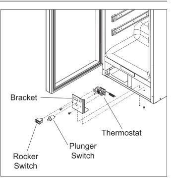
Figure 5-8. Light Switch, Plunger Switch and Thermostat Removal
