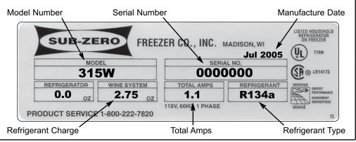
Figure 1-2. Serial Tag Layout
