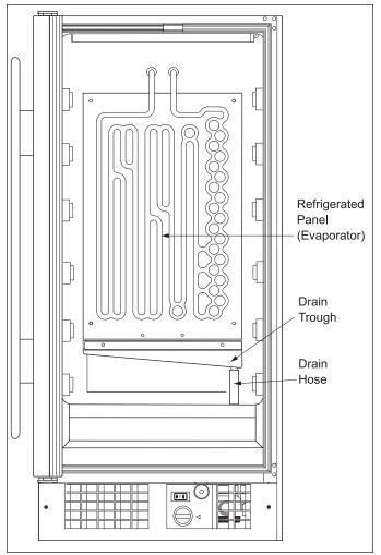
Figure 3-7. Drain System
