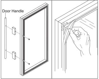
Figure 5-2. Door Handle and Gasket Removal
