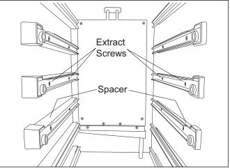
Figure 5-10. Slide and Spacer Removal
