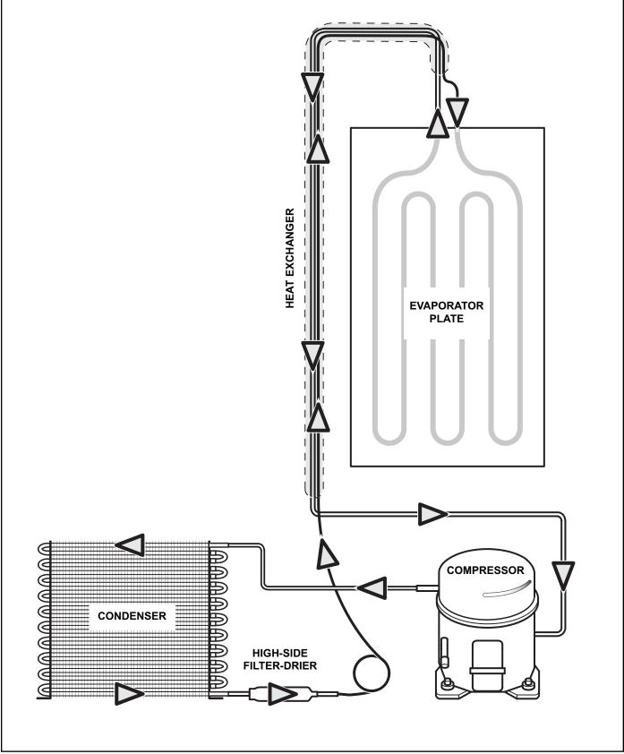
Figure 4-7. Model 315W Refrigerant Flow
