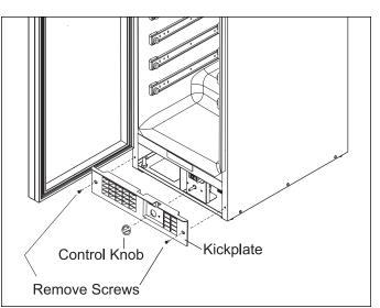
Figure 5-1. Kickplate Removal
