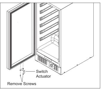
Figure 5-4. Light Switch Actuator Removal
