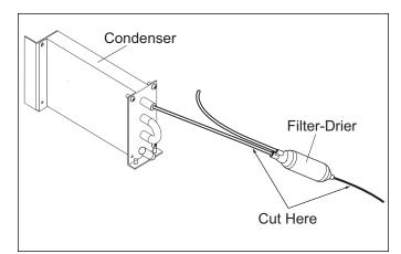
Figure 5-15. Cut Drier Inlet & Outlet
