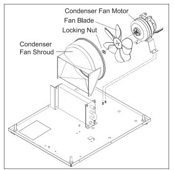
Figure 5-12. Condenser Fan Motor Removal
