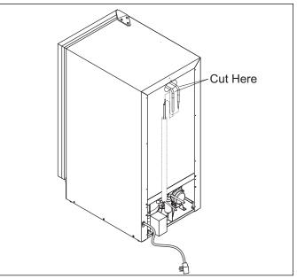
Figure 5-13. Cut Heat Exchanger
