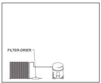
Figure 4-3. Filter- Drier
