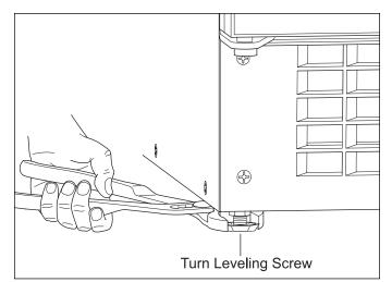
Figure 2-5. Unit Leveling
