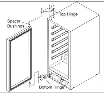
Figure 5-3. Door and Hinge Removal
