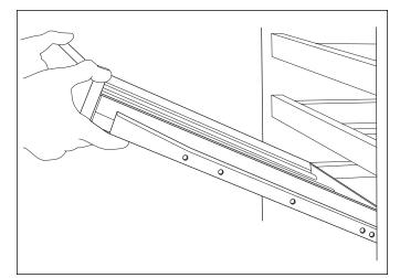
Figure 5-9. Wine Rack Assembly Removal
