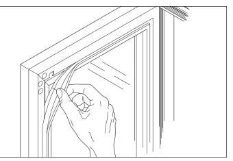
Figure 3-4. Door Gasket Removal
