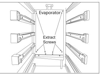
Figure 5-14. Evaporator Removal
