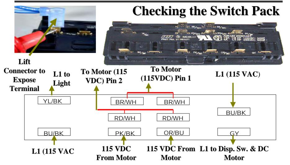
Crushed Ice Switch = Continuity from OR/BU (com) to RD/WH wires, and PK/BK (com) to BR/WH wires.
