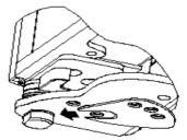
Turn the bushing located underneath the bottom of the hinge using the open-end wrench. Turning the bushing to the left (counterclockwise) will raise the door. Turning the bushing right (clockwise) will lower the door.
