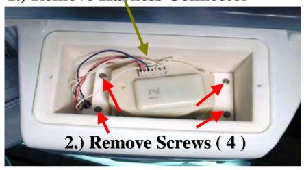
Use care not to pinch or damage the harness during motor removal or reassembly
