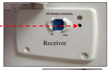
Door opens to block the light beam indicating the Freezer door is open or the ice bucket is missing
