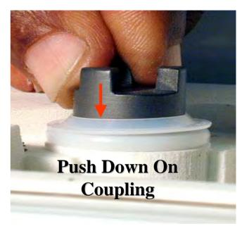
**Push Drive Shaft into Motor**
