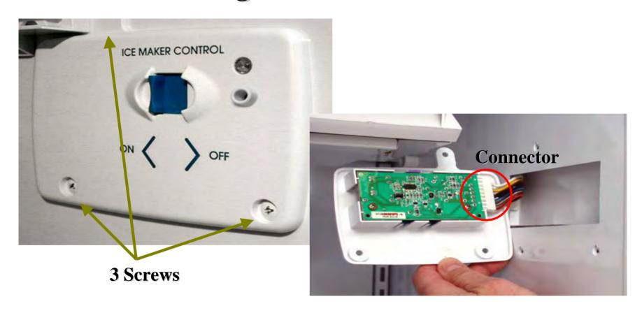
Reminder: Safe repair practice requires disconnecting the power before servicing any electronic control boards
