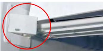
If the Receiver does not "see" the light from the Transmitter the Icemaker power is shut off and no ice will be harvested
