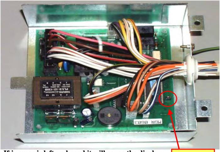
If jumper is left on board it will cause the display to go into the test mode when unit is powered up.
