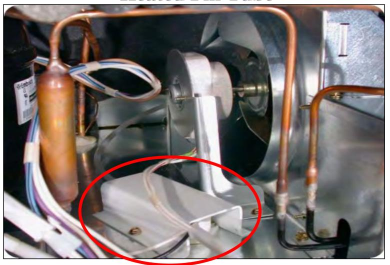
The heated fill tube is energized for 90 minutes after each icemaker fill
