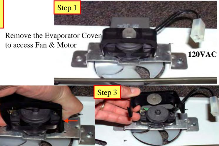
Squeeze rear motor bracket to release it from the front bracket
