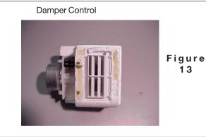
When the food compartment control calls for cooling, the contacts in the control will close sending a signal to the ADC. The ADC then will start the damper motor running to open the damper. (See Figure 14.)
