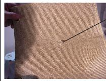
Cut a small hole in the middle of the shield.
