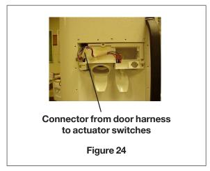
The original heater for the ice chute and housing are foamed in place with the one piece door. It is connected to the door wiring (See Figure 25) harness by a plug coming out of the inner door panel with 2 black wires connected to it. (See Figure 25) If the heater fails, it will be necessary to install an external heater on the housing chute opening in place of the internal heater. The replacement heater will connect to the same plug as the original heater. (See Figure 26)
