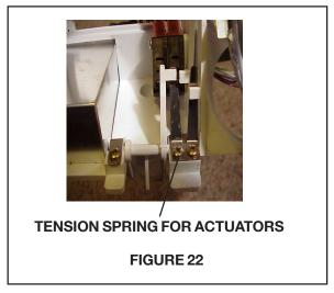
The Actuators are held in place by stainless clamps at each end of the actuator and the two bladed spring in the middle. (See Figure 23) The actuators can be removed by removing the 4 screws and lifting the paddle / ice chute out of the housing.
