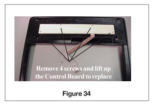
Current will be carried between the power board and the control board by a ribbon connector (See Figure 35). You can check the wires with a ohm meter if you suspect a broken wire.
