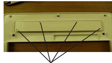
Remove 4 screws and lift up the Control Board to replace
