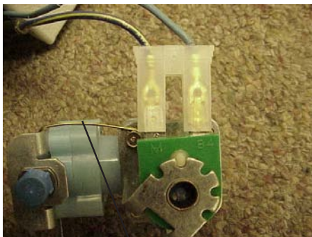
Terminal on Coil is Installed Over Top of Terminal on Left Side of Plug
