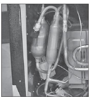
Figure 7-16. Two Stage Drier Kit
