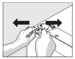
**3** Detach the water tube from the connector located behind the refrigerator and pull the tube back out to the front of the unit. The connector releases when you press inward on the outer sleeve while pushing the tube toward the connector then while continuing to hold in the sleeve, pull the tube away.
