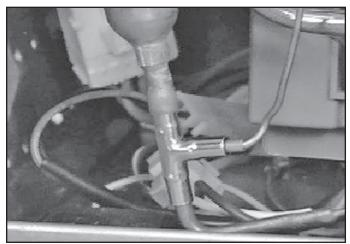
Figure 7-15. Dye Drier Kit
