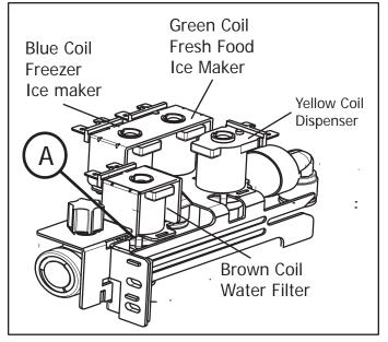
Figure 5-1. Water Valve (Dispenser Model Shown)
