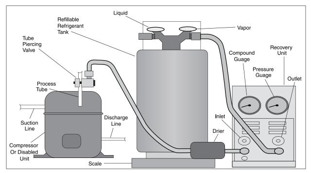
Figure 7-4. Installation of Recovery Equipment
