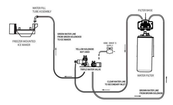
Note: Some non-dispenser models are constructed with a single water valve.
