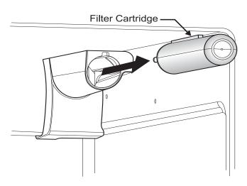
Figure 5-3. Removing Water Filter Cartridge
