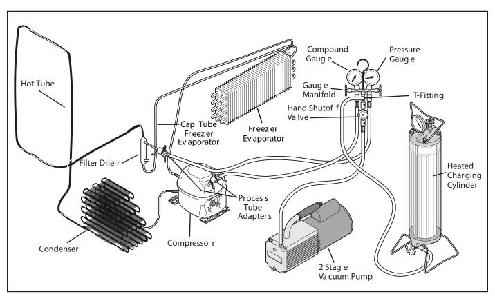
Figure 7-23. Installation of Recovery Equipment Non-Dispenser
