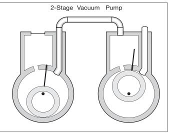
Figure 7-24 Two Stage Vacuum Pump
