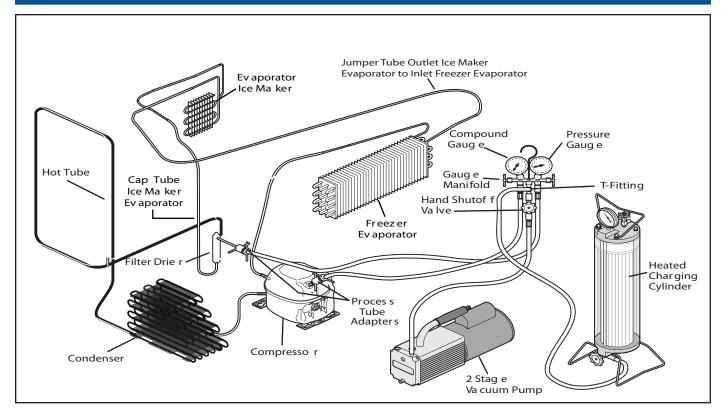
Figure 7-22. Installation of Recovery Equipment Dispenser with Flex Tray Ice Maker
