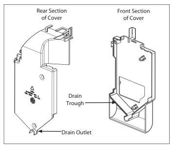
Figure 4-10. Icemaker Water Drain
