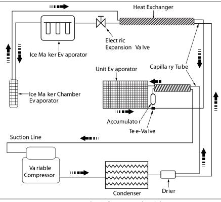
Figure 4-11. Ice Maker Refrigeration Flow Schematic
