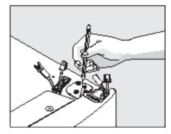
2 Disconnect the harness by grasping both sides of the connector firmly, depress the latch, and pull apart. Remove the two (2) screws from the top hinge. Lift the door off of the bottom hinge and set it aside.
