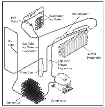
Figure 4-9. Ice Maker Refrigeration Schematic
