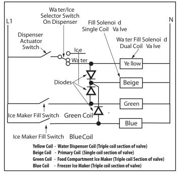
Figure 5-2. Diode Schematic
