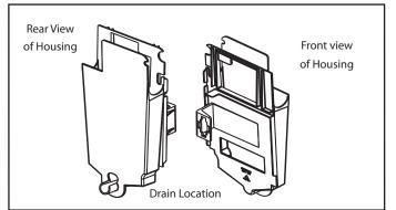
Figure 4-6. Evaporator Cover and Drain
