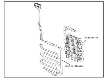
Figure 4-4. Evaporator and Defrost Heater
