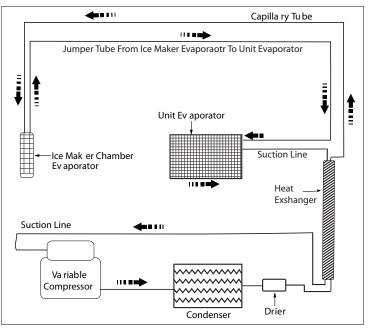
Figure 4-7. Ice Maker Refrigeration Flow Schematic
