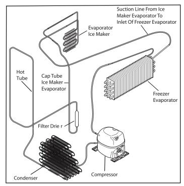
Figure 4-2. Ice Maker Refrigeration Schematic
