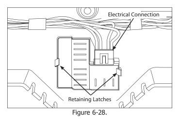
**NOTE:** The humidity sensor is mounted on the control board for the non-dispensing models. Failure of the humidity sensor for those models requires replacement of the control board.
