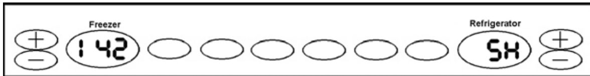
FAIL RESULT - Thermistor is shorted
