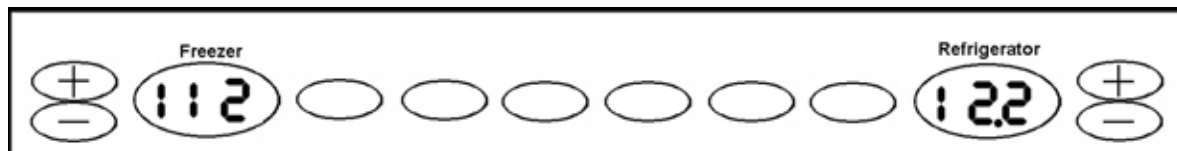
EVAPORATOR FAN IS ON
