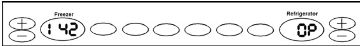
FAIL RESULT - Thermistor is Open
