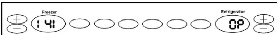
FAIL RESULT - Thermistor is Open
