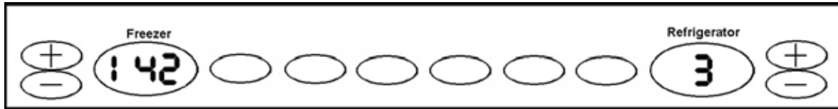
PASS RESULT – Displaying the Temperature inside Freezer
