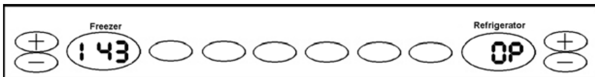
FAIL RESULT - Thermistor is Open
