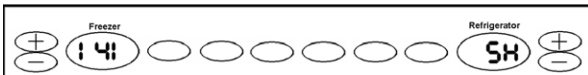
FAIL RESULT - Thermistor is shorted
