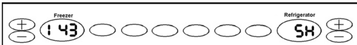
FAIL RESULT - Thermistor is shorted
