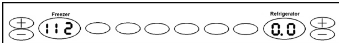
EVAPORATOR FAN IS OFF
