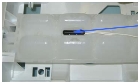
Icemaker sensor located under insulated pad.
