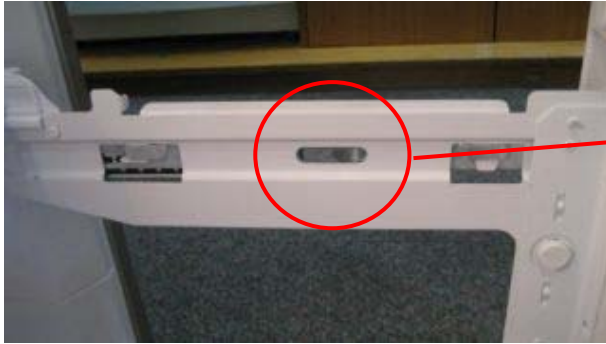
Push Locking Tab in to release bracket from slide.
