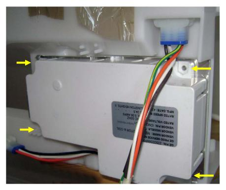
Remove 4 mounting screws and nuts located in the 4 corners.
