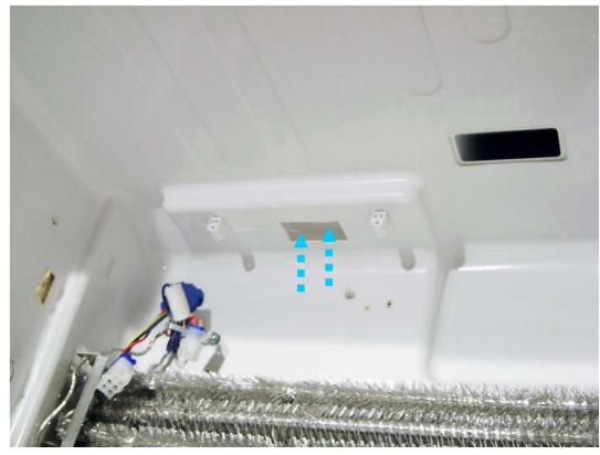
Freezer air travels up through channel and into ice door section
