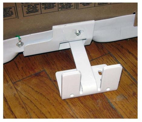
Anti-tip bracket mounts to floor or wall
