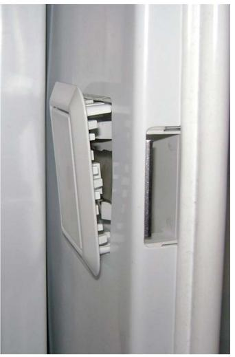
Pry gently around the lip of the cover with a small screwdriver to remove
