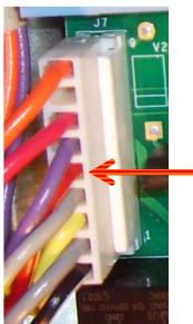
Port heater cycles based on temperatures and ice box condition. (Ex: mid –mid settings appx 30% on time.) Test from J7 – 9 (Orange neutral) to J7 – 5 (Red/Ylw)
