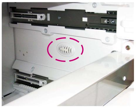
FF Thermistor located on top left side wall Tested at J1 connector of main board FZR Thermistor located on right side wall Tested at J1 connector on main board
