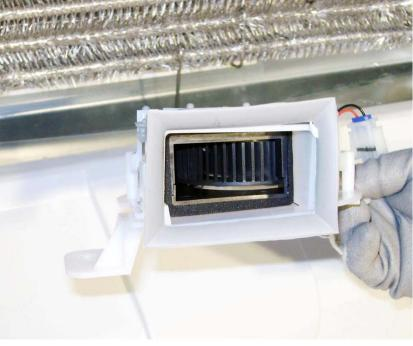
Blower comes as an assembly Rubber boot separate part.
