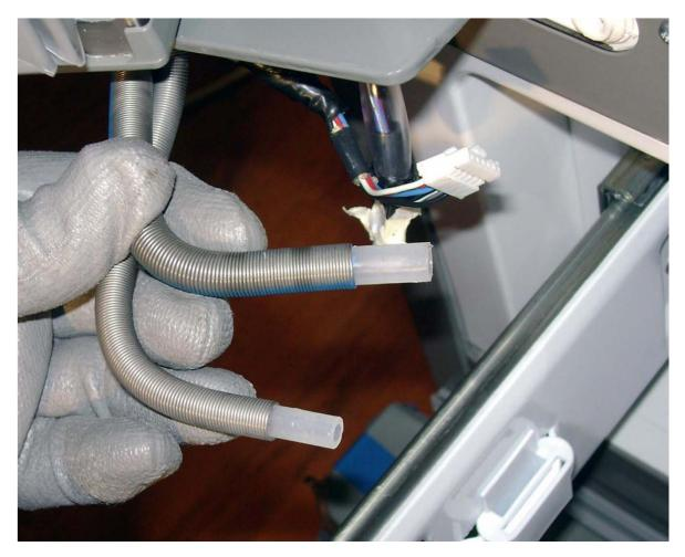
**NOTE**: Water line is larger diameter than IM line
