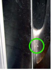
3/32 Allen screw for handle removal
