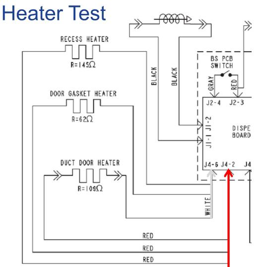
Heaters operate based on temperature settings i.e. FRZ setting of 5 or higher = 100% "On" time except during ice dispense. (Circuit can be tested at dispenser board also. Wh/Red)
