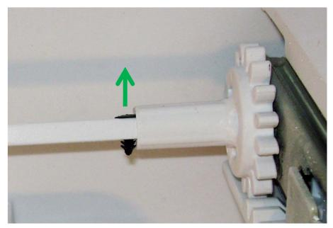
To remove side wall tracks, start by removing the roller guide bar. Remove small black locating pin and slide bar to right and remove from rollers.
