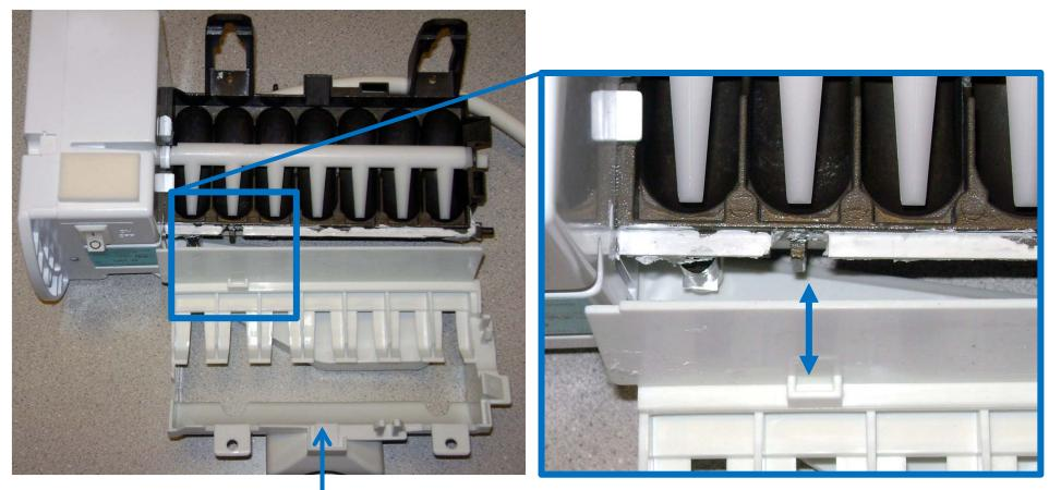
Note fill cup assembly removed and upside down for better viewing.
