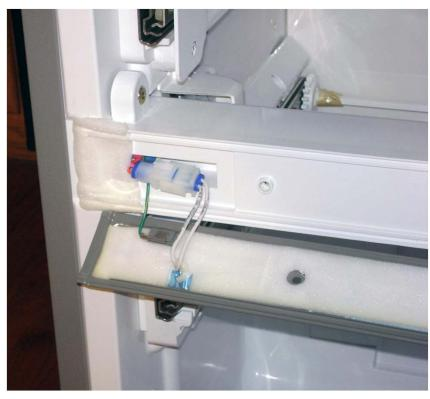
Remove 4 screws securing mullion heater and face plate.
