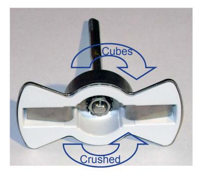
Clockwise - Cubes Counter-clockwise - Crushed (Facing bucket)
