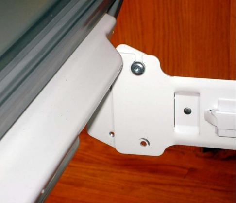
Remove outer panel by removing the lower T30 torx screw. Loosen the top one and lit panel up and off.
