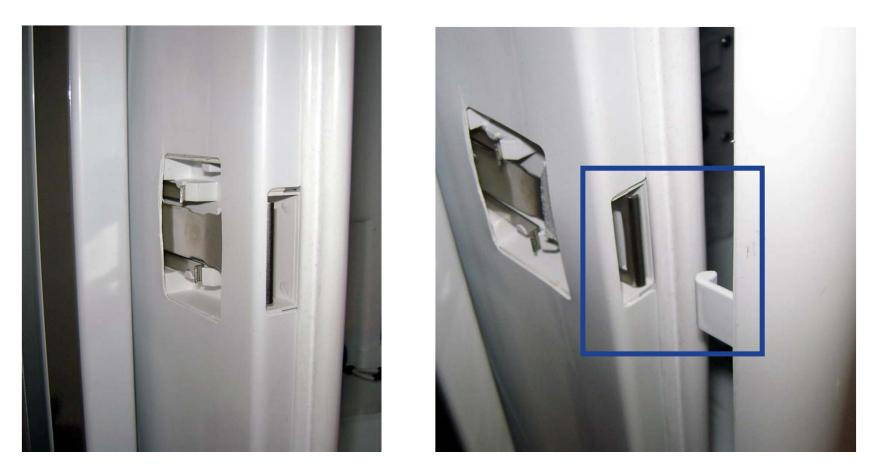
Simple design as metal "catch" bends in and out to secure and release door strike
