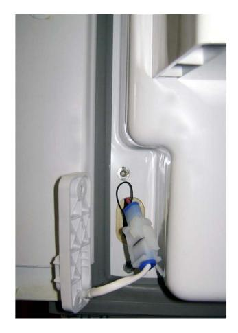
Check heater for 24  $\Omega$  resistance or 13 VDC (voltage only present if heater should be on)
