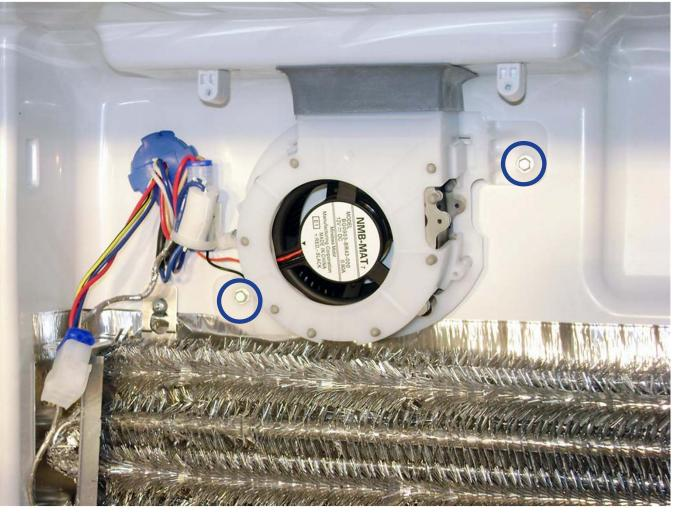
Disconnect plug. Remove two ¼ hex head screws to remove blower
