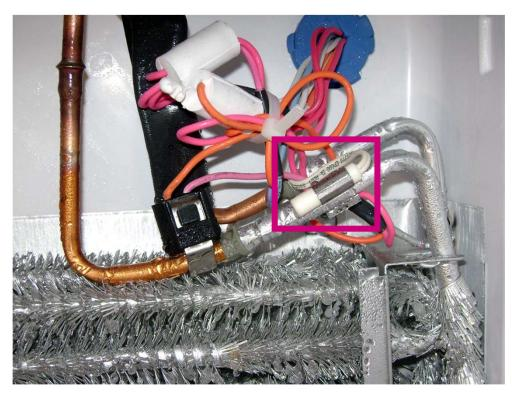
Evaporator thermistor clipped to tubing.
