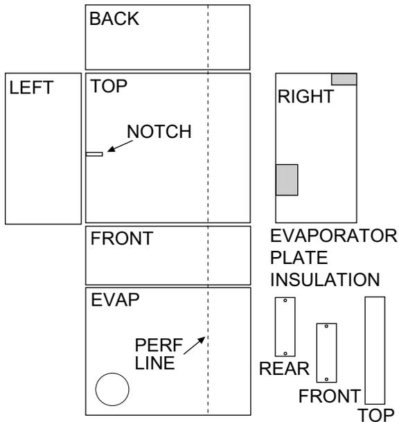
Insulation pieces to cover entire evaporator compartment
