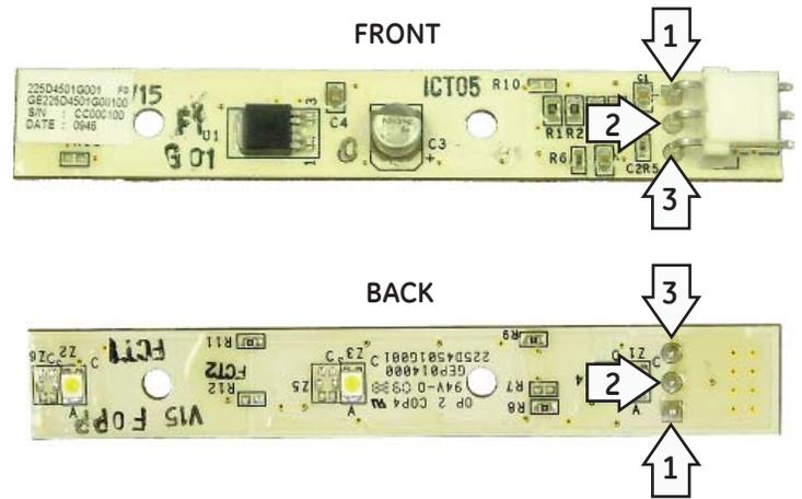
The LED board is defective if both DC voltages are present and the LEDs are not lighting. These boards can also be swapped for testing.
