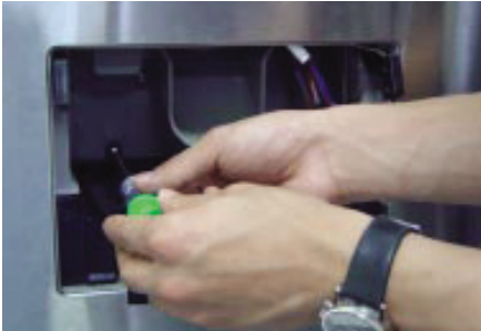
7) Unscrew 2 points to separate tray-cover
