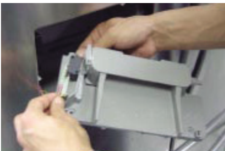
12) Separate the Switch connection harness.
